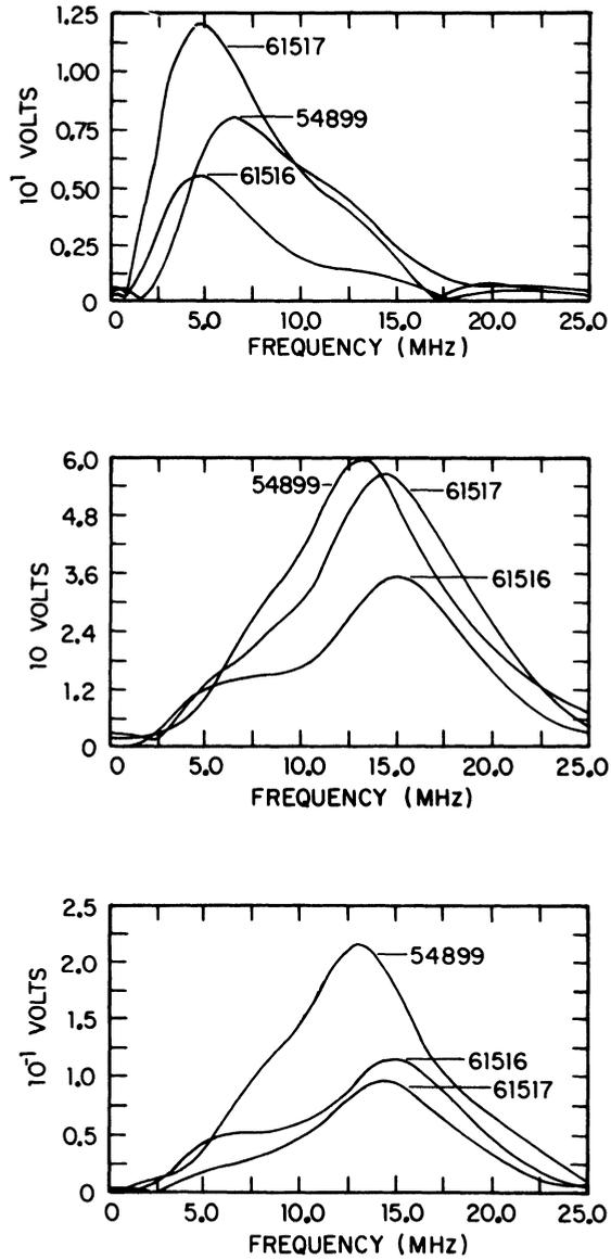
Fig. 2. Spectral response from back surface of three host materials for three transducers.
