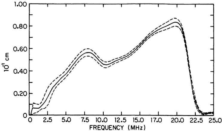
Fig. 5. Corrected scattering amplitude for transducer 61516 with titanium showing mean  $\pm 1$  standard deviation for 9 independent experiments.
