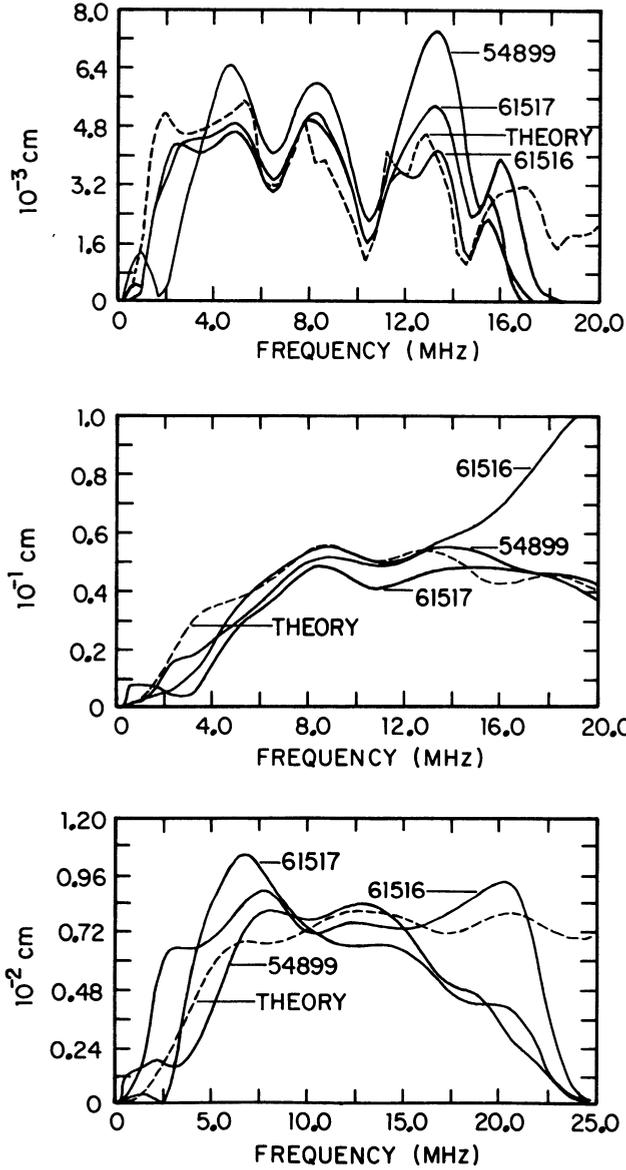
Fig. 4. Corrected scattering amplitude from three samples and three transducers.
