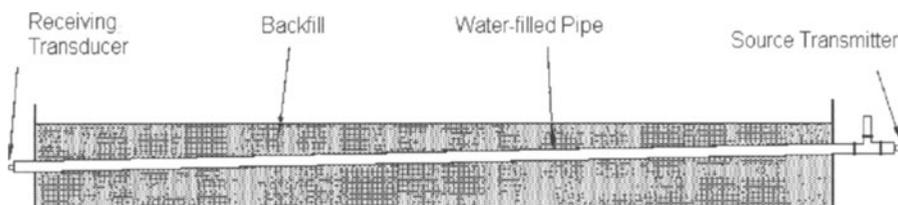
Figure 1: Backfill Experimental Apparatus.
