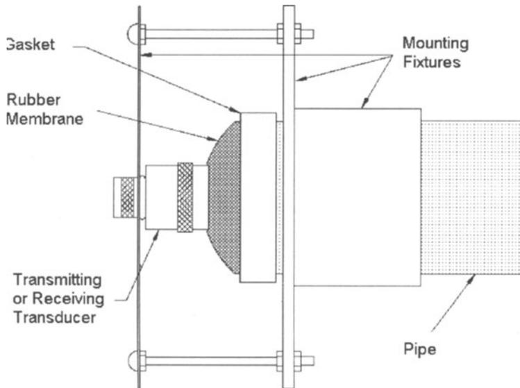
Figure 2: Transducer mounting setup.
