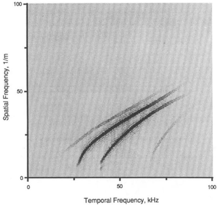
Figure 5: Axi-symmetric dispersion characteristics in a model pipeline (10 PD to source)<sup>2</sup>.
