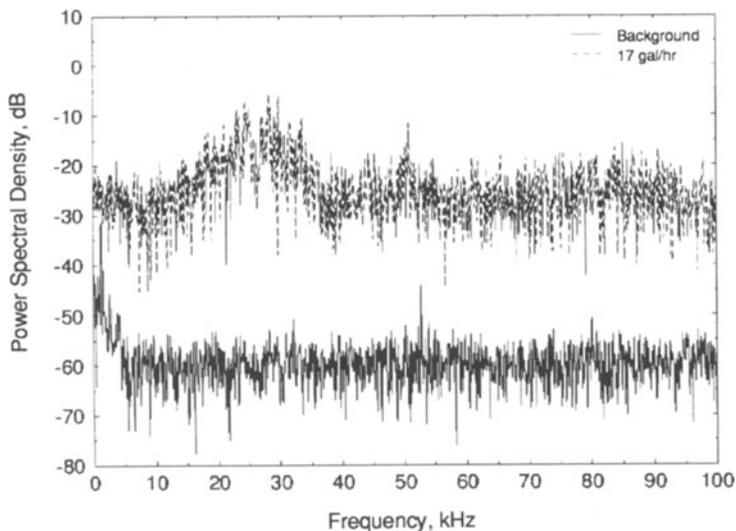
Figure 4: Spectra of leak signal produced by sand-covered leak source. Receiver approximately 20 ft. from source location<sup>1</sup>.
