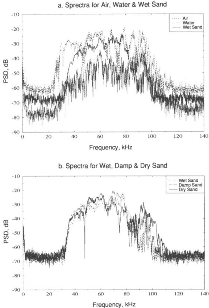
Figure 3: Received spectra as a function of backfill.
