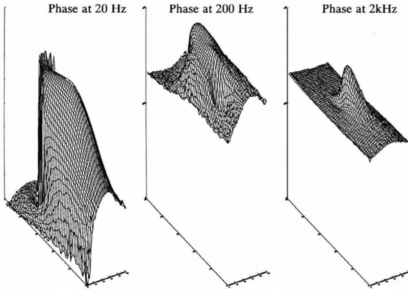
Figure 5. Phase plots for the 1.27 mm thick aluminum specimen.
