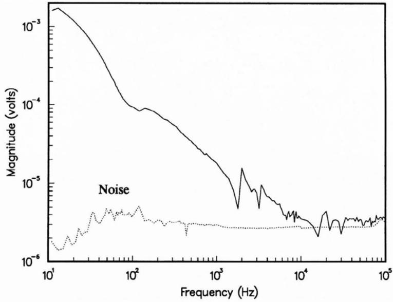
Figure 3. Thermal-Acoustic signal as a function of frequency for a 1.27 mm thick aluminum specimen.
