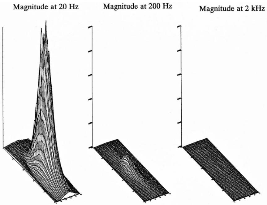
Figure 4. Magnitude plots for the 1.27 mm thick aluminum specimen.
