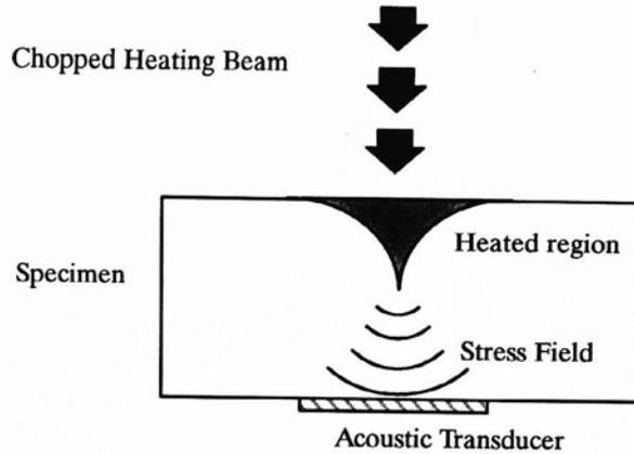
Figure 1. Thermal-Acoustic Effect.
