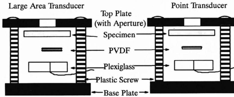
Figure 2. Conventional large area and point TA transducers (Exploded view ).
