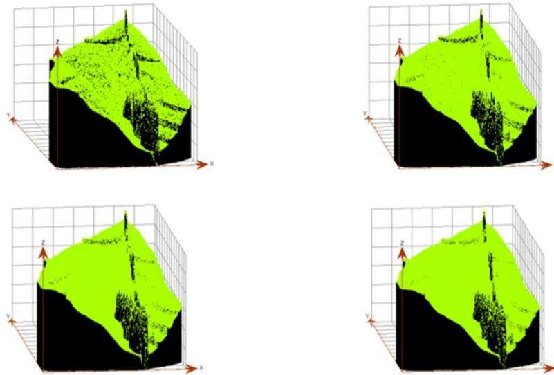
**Figure 2:** Overview of altimetry data by LiDAR Cloud of a small hydrographic basin of the region of the town of Treynor - Iowa – USA with 25% of the data (upper left), 50% (upper right), 75% (lower left) and 100% (bottom right).
