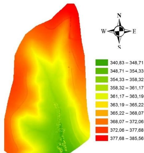
**Figure 5:** Simple Kriging of altimetry data, obtained by LiDAR Cloud, of a small hydrographic basin of the region of the town of Treynor - Iowa - USA.
