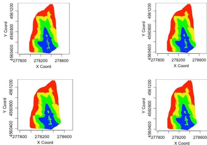
**Figure 3:** Data behavior presentation about the "intensity" of altimetry obtained by LiDAR Cloud of a small hydrographic basin of the region of the town of Treynor - Iowa - USA, using the graphic of quartiles. 25% of the data (upper left), 50% (upper right), 75% (lower left) and 100% (bottom right).
