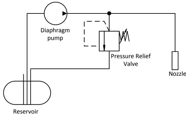
Figure 2. Schematic of hydraulic circuit used for metering liquids to the nozzle
