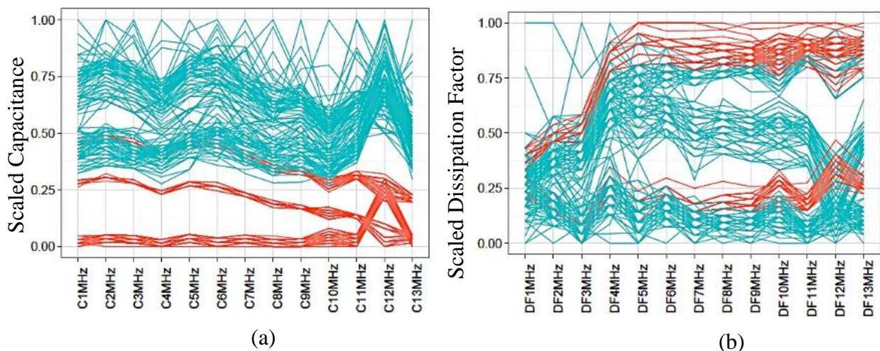
**Figure 4. (a) Capacitance and (b) dissipation factor values scaled to minimum zero and maximum one for spray (blue lines) and no-spray (red lines) cases across multiple frequencies for tests with deionized water.**
