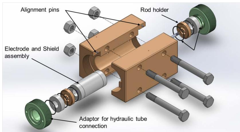
Figure 3. Exploded view showing flow-through design of the sensor and arrangement of different metallic parts and dielectric assembled
