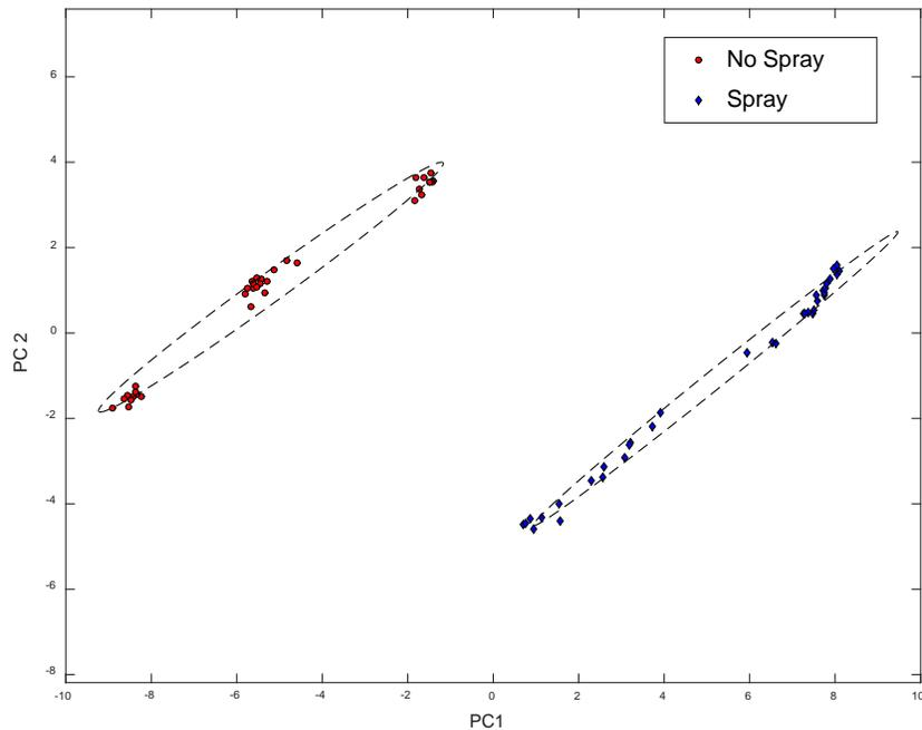
**Figure 7. Dielectric spectroscopic data from the test with oil projected onto the first two principal components. Red and Blue represent data points for no-spray and spray cases respectively.**
