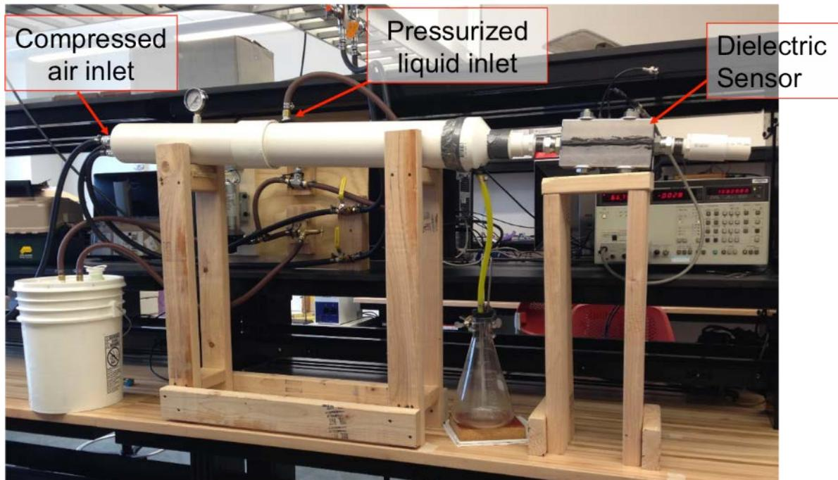
**Figure 1.** Experimental apparatus used for the test with deionized water shows the hydraulic circuit and impedance analyzer used for the test.
