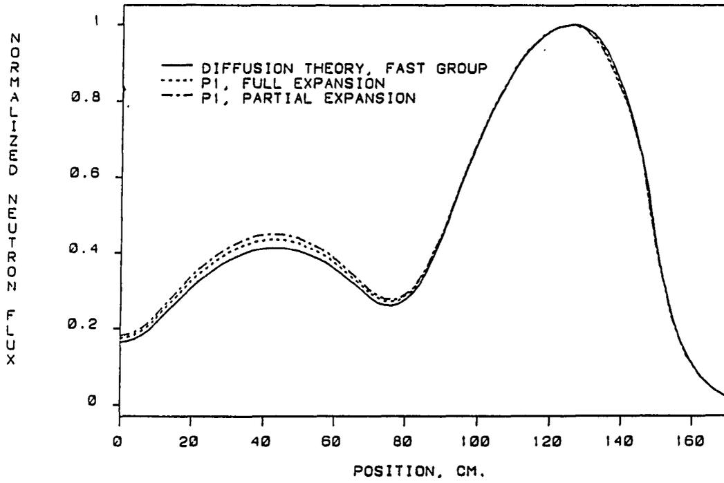
Figure V-2. Fast flux profiles for sample problem one
