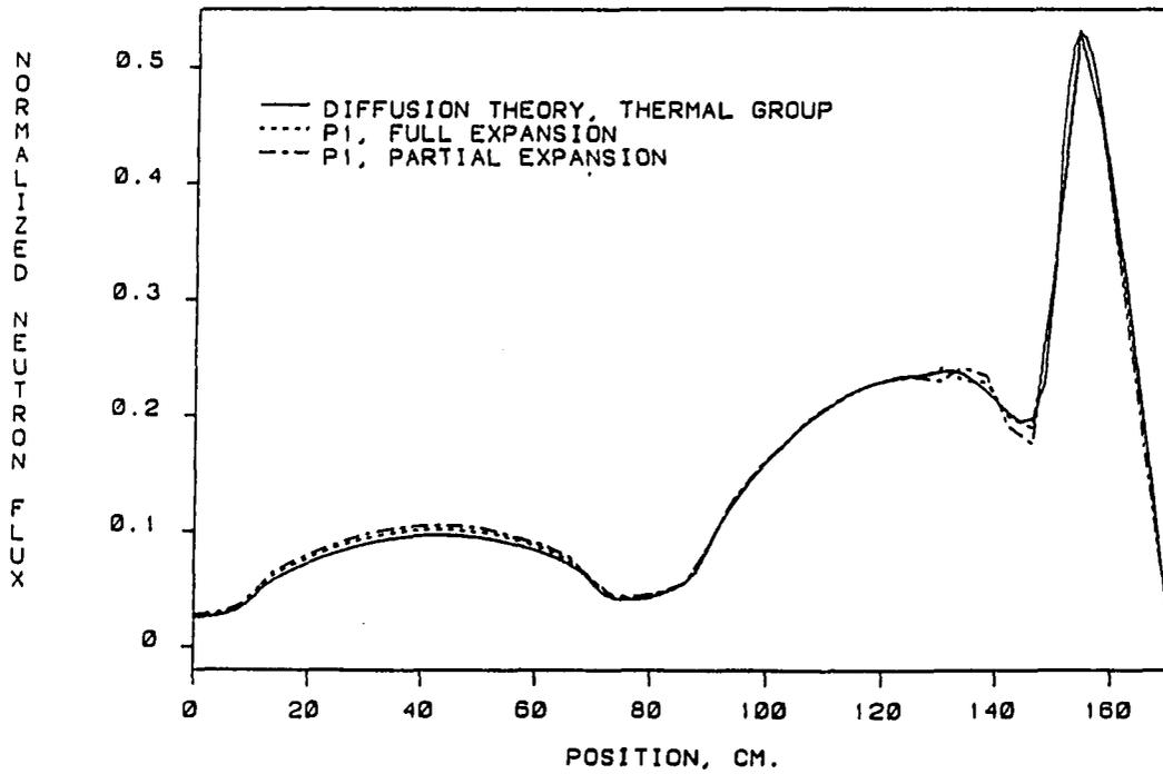
Figure V-3. Thermal flux profiles for sample problem one
