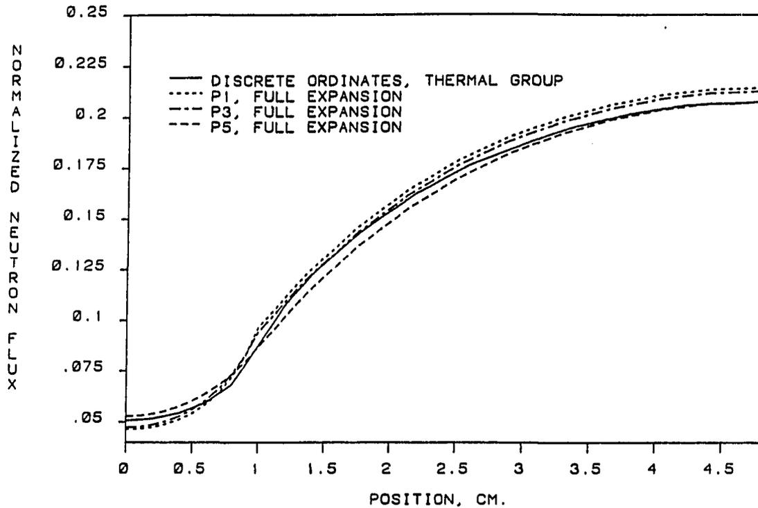
Figure V-11. Thermal flux profiles for sample problem two
