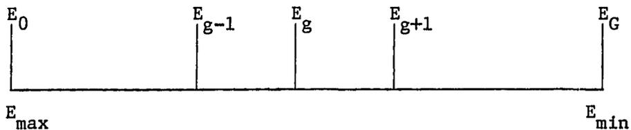
Figure III-1. Multigroup partitioning of the energy range
