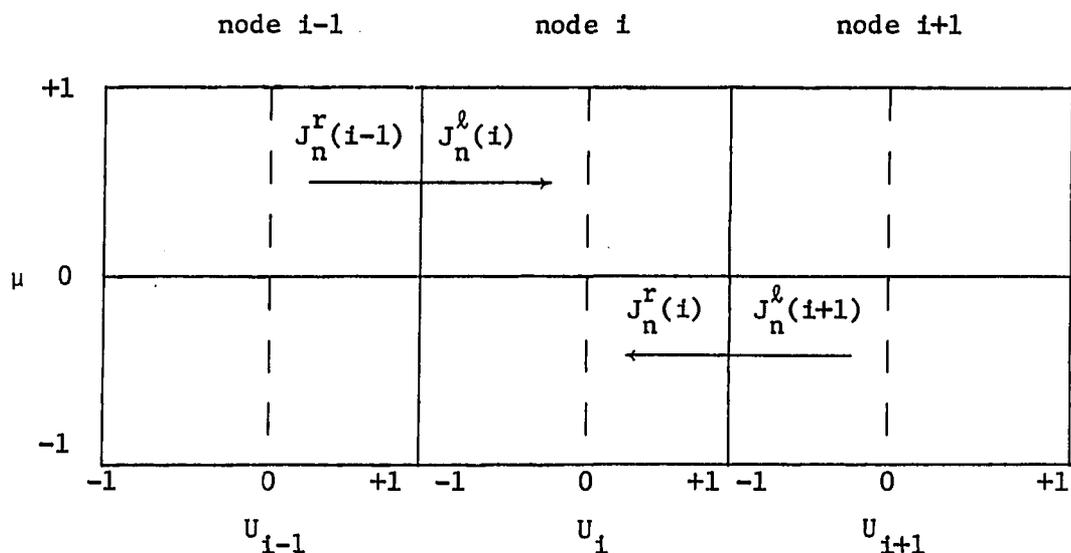
Figure IV-2. Interface conditions for the nodal geometry
