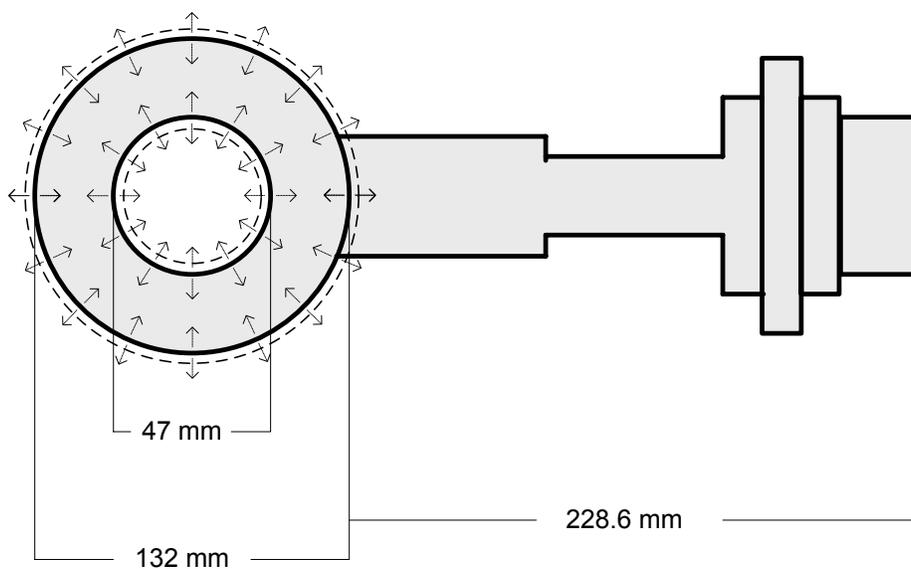
**Figure 2. Branson ultrasonics "donut" shaped horn**
