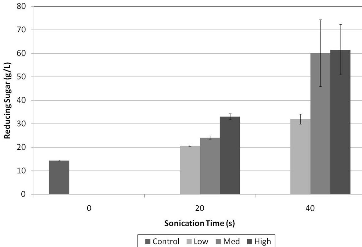
**Figure 3. Reducing sugar yield of ultrasonic batch system**
