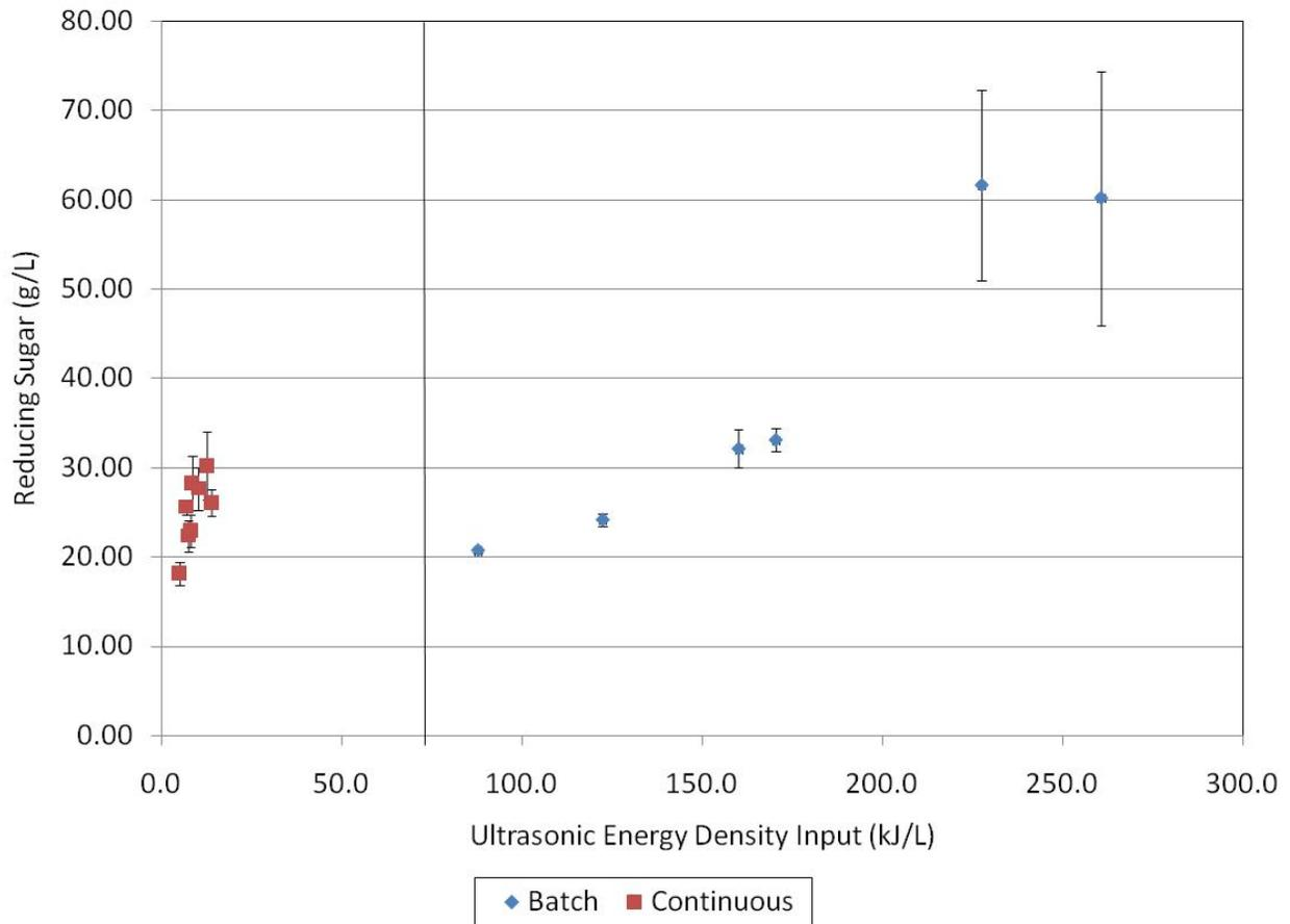
**Figure 10. Reducing sugar yield of corn slurry as a function of ultrasonic energy density input**
