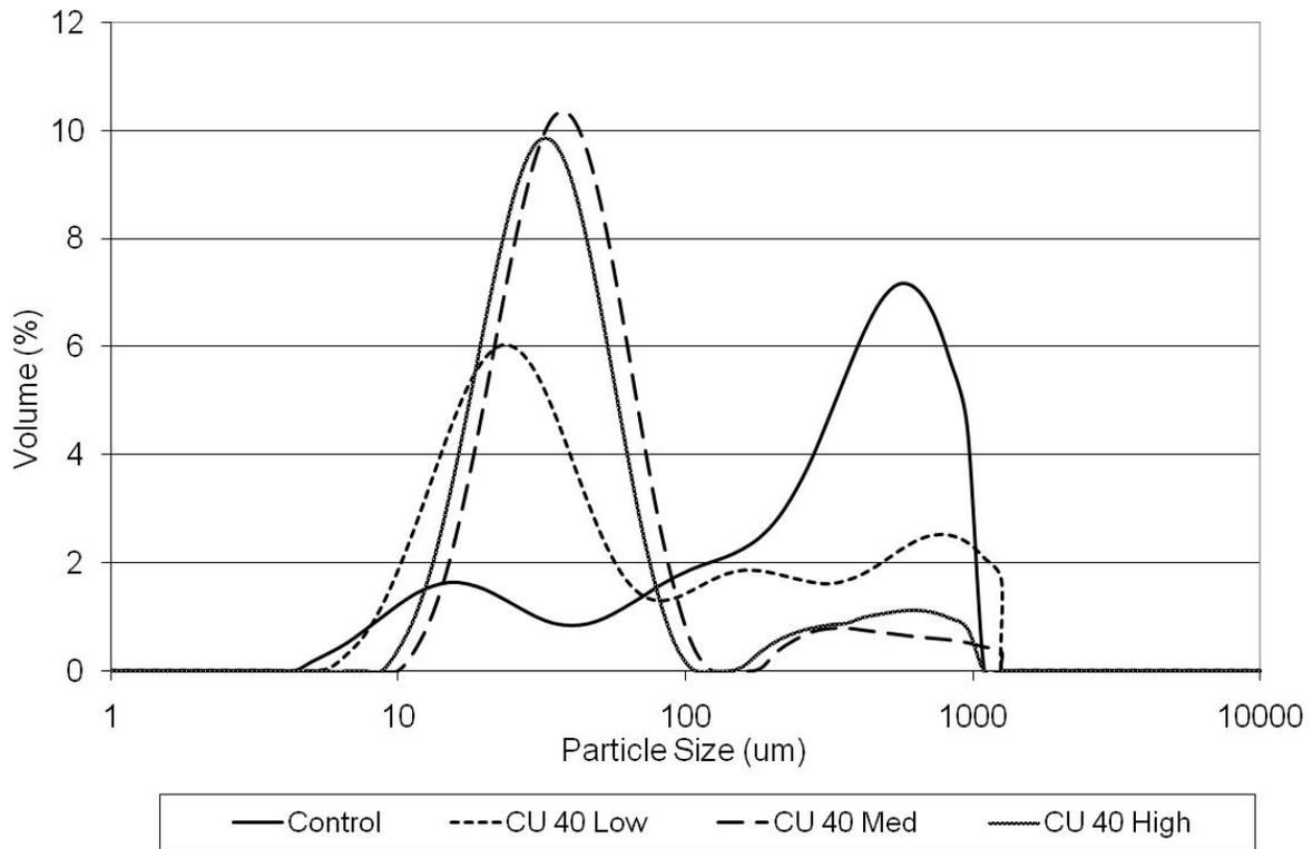
**Figure 6. Particle size analysis of ultrasonic batch systems at varying power input for 20s sonication time**
