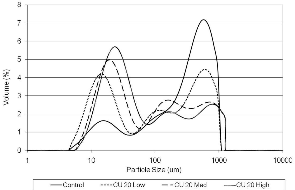
**Figure 5. Particle size analysis of ultrasonic batch system at varying power input for 40s sonication time**
