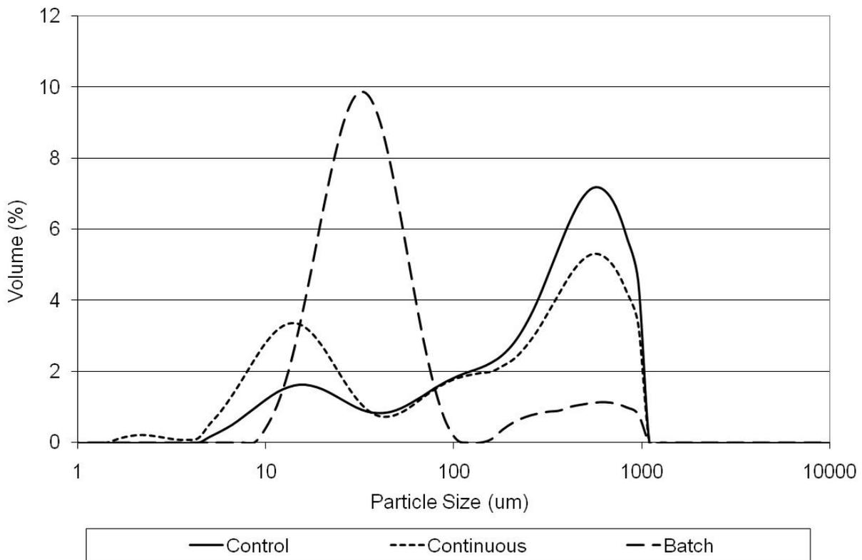
**Figure 8. A comparison of the particle size analysis of ultrasonic batch and continuous systems**
