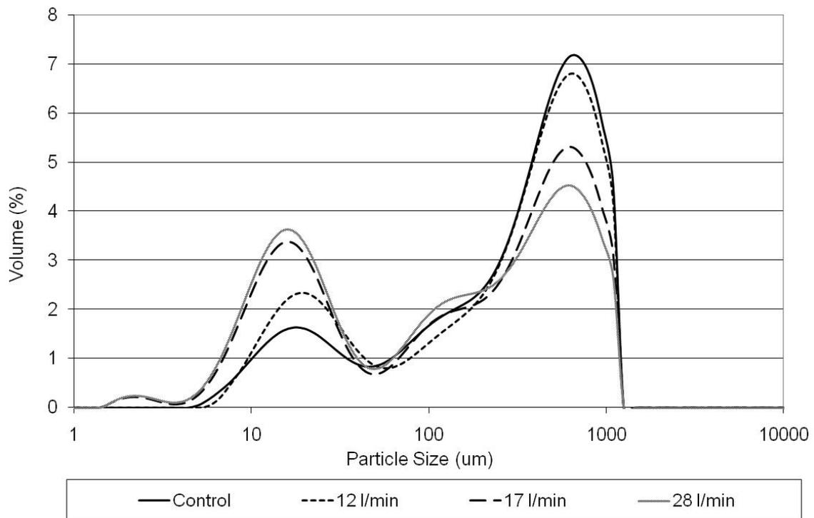
**Figure 7. Particle size analysis of ultrasonic continuous systems at varying flowrate**
