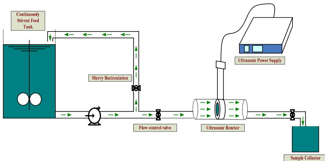
**Figure 1. Ultrasonic continuous system experimental set-up**
