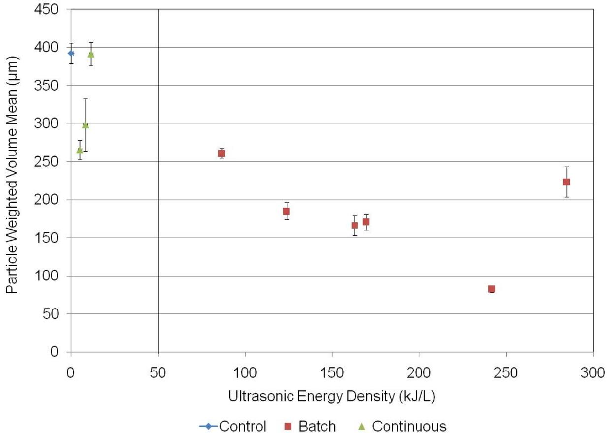
**Figure 9. Effect of ultrasonic energy density on the particle weighted volume mean**
