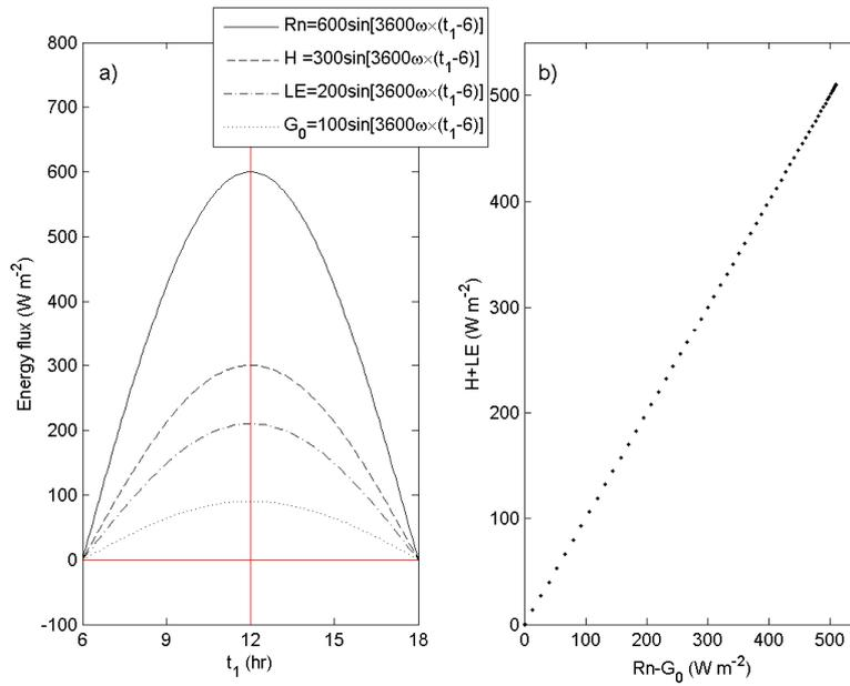
**Fig. 2.** Theoretical demonstration of (a) temporal variations in surface energy components ( $Rn$ ,  $H$ ,  $LE$ , and  $G_0$ ) during daytime, and (b) comparison between turbulent heat fluxes ( $H+LE$ ) and surface available energy ( $Rn-G_0$ ).
