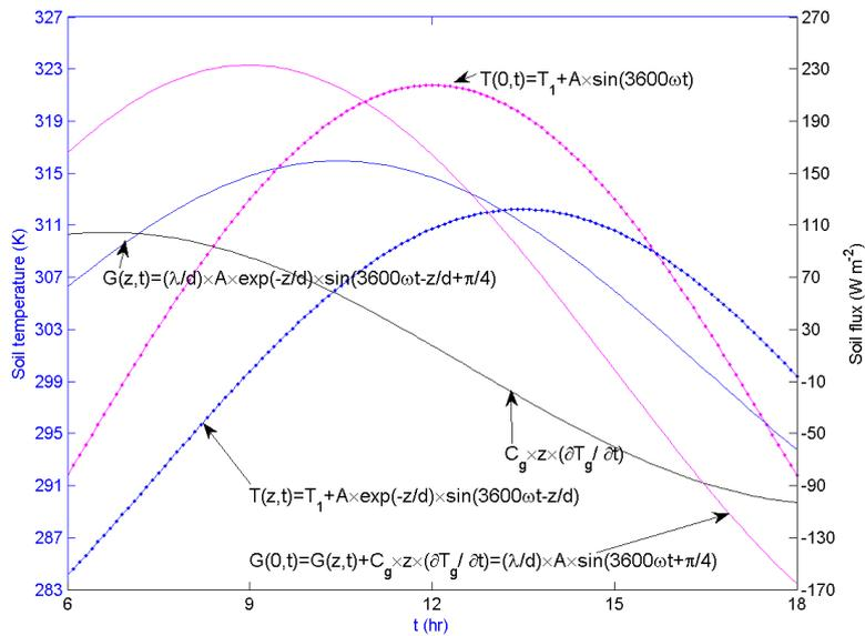
**Fig. 1.** Theoretical demonstration of temporal variations in soil surface temperature  $[T(0, t)]$ , soil temperature  $[T(z, t)]$ , soil surface heat flux  $[G(0, t)]$ , soil heat flux  $[G(z, t)]$ , and soil heat storage  $C_g z \partial T / \partial t$  during daytime.
