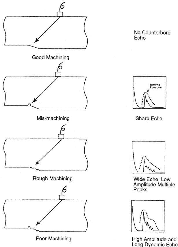
Fig. 4. Examples of various counterbore conditions.
