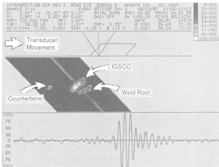
Fig. 3. Example B-scan presentation showing the axial separation between root and crack indications.
