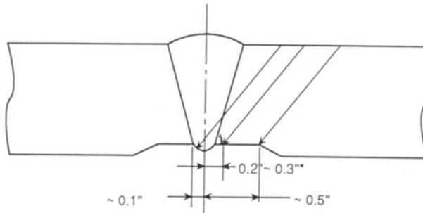
\* The distance depends on wall thickness and welding condition
