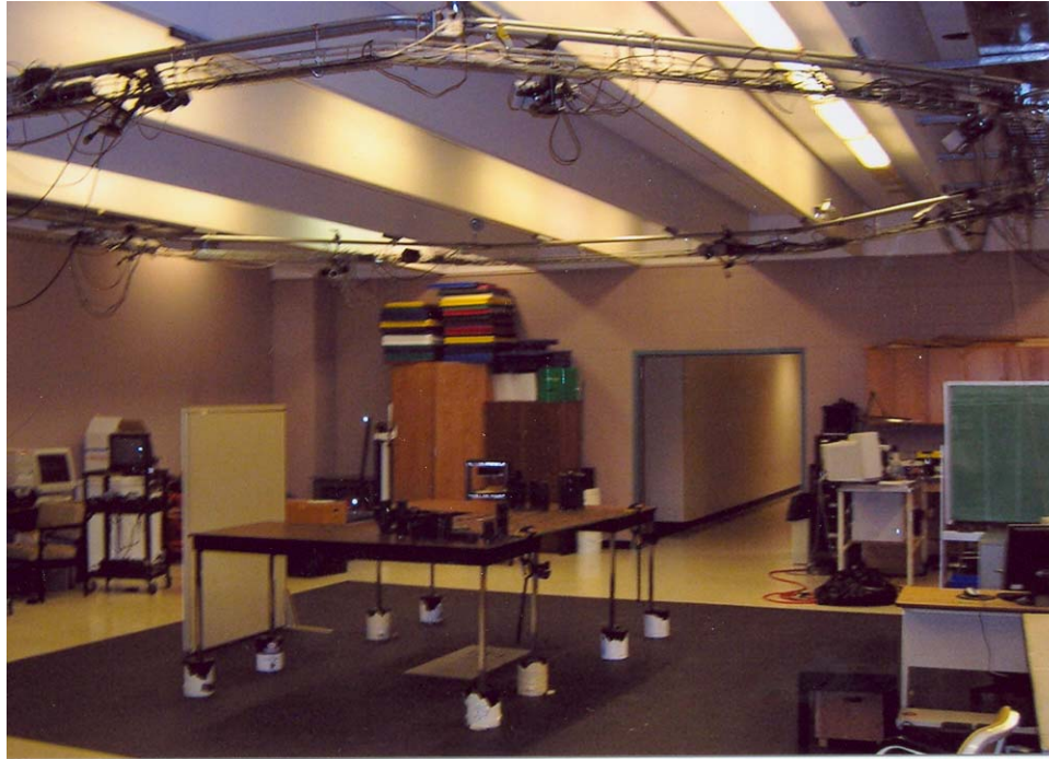
Figure 9: Scanning table and eight octagon camera system with seven cameras visible
