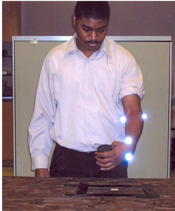
Figure 7: Flexion/extension—subject in flexion plane with four of five markers visible
