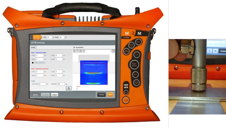
Figure 1. Ultrasonic probe over a resistance spot weld part (left) and display of the cross-section ATFM image (right) within a portable phased array system.
