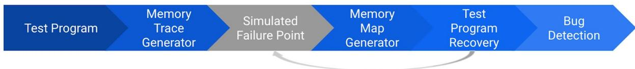
Figure 3: Test Framework Layout
