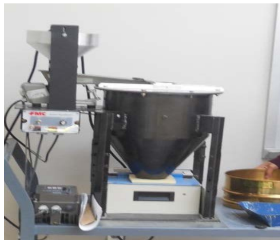
Figure 2. Insect fragments quantification from wheat samples using a laboratory scale Entoleter.
