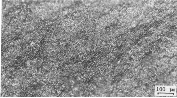
Fig. 6. Fracture surface of sample bonded at 600°C for 4 hours.
