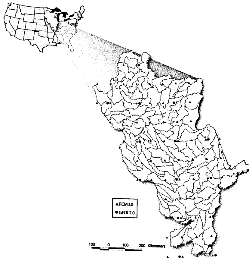
Figure 1: Location of the study domain (Upper Mississippi River Basin), subbasin delineation for SWAT simulations, and spatial resolution of climate model grid/data points.
