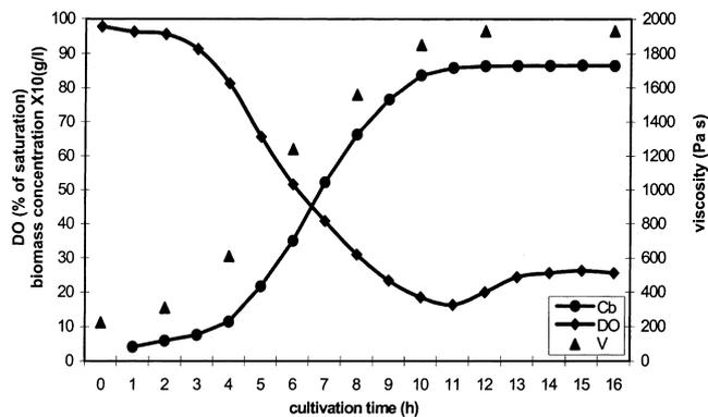
Figure 2. Profiles of mycelial biomass concentration ( $C_b$ ), viscosity ( $V$ ) and DO level of culture broth as a function of the cultivation time.
