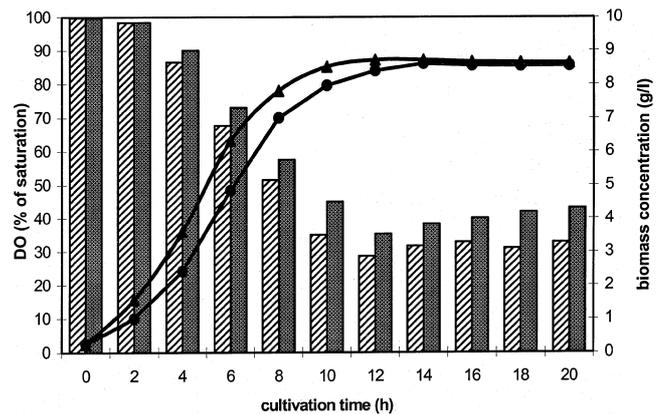
Figure 6. Profile of mycelial biomass concentration ( $C_b$ ) and DO level during the cultivation of *R. oligosporus* using TEALB with single and double sparger air supply.
