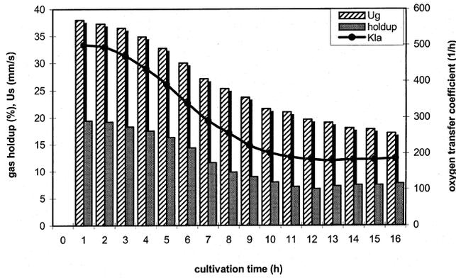
Figure 3. Hydrodynamic profiles of gas holdup, superficial gas velocity ( $U_g$ ) and oxygen transfer coefficient ( $K_{La}$ ) as a function of the cultivation time.
