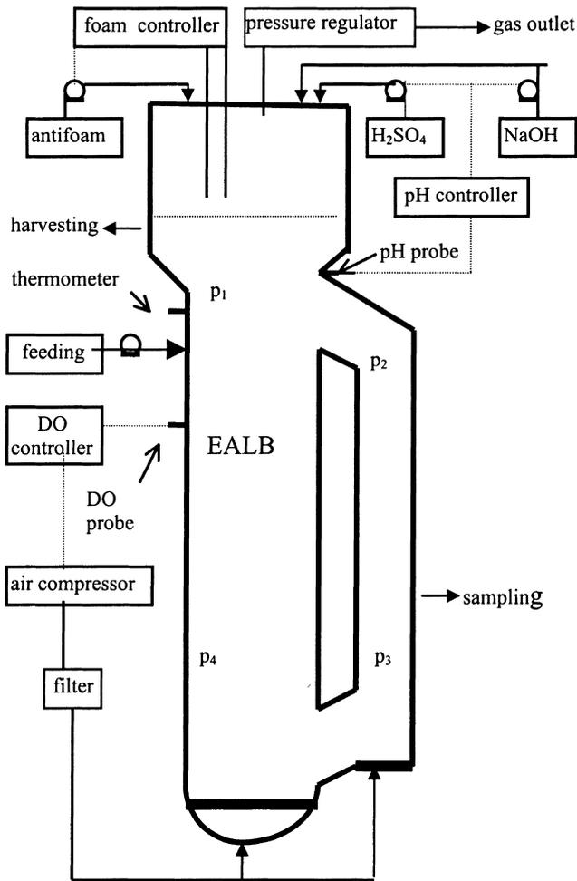
Figure 1. Schematic diagrams of the experimental set up ( $p_1$ ,  $p_2$ ,  $p_3$  and  $p_4$  – positions of pH probes for testing pulse tracer).
