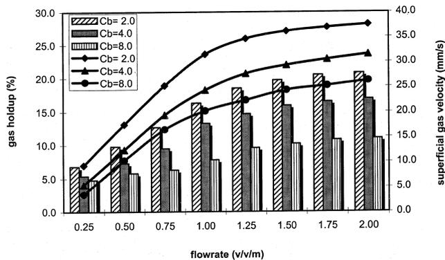
Figure 4. Effect of air flow rate and mycelial biomass concentration ( $C_b$ ) on gas holdup (column) and superficial gas velocity (line).
