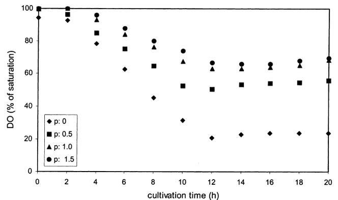
Figure 7. DO profiles during the mycelial cultivation process with top pressure ( $P$ ) operations.
