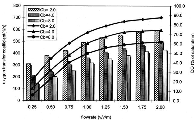
Figure 5. Effect of air flow rate and mycelial biomass concentration ( $C_b$ ) on oxygen transfer coefficient (column) and DO level (line).
