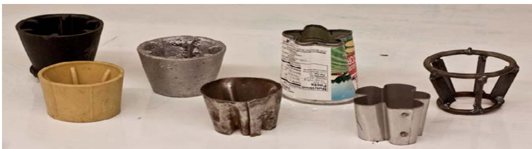
Figure 9. Different types of local maize shellers (MIT, 2015)
