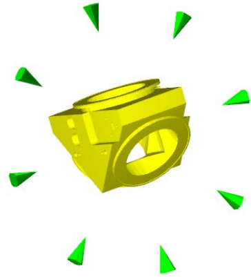
Figure 10. The main block model which requires many setups to machine every facet.
