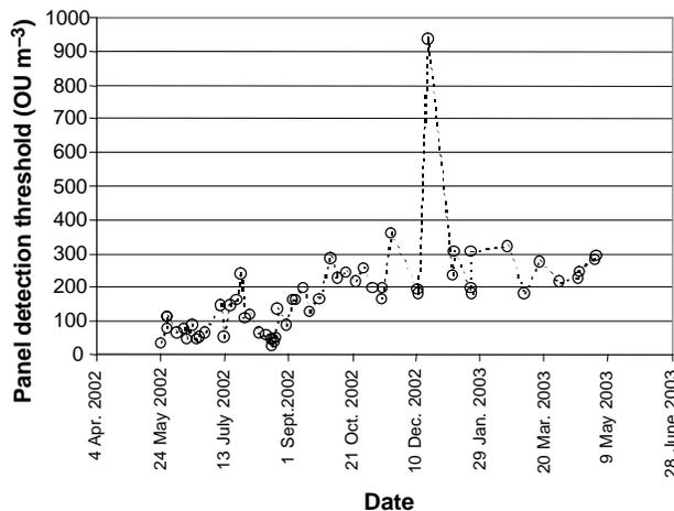
Figure 1. Panel detection thresholds determined for a bag filled with 40 ppm n-butanol standard gas.
