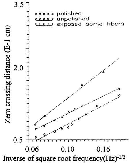
Figure 4. Zero crossing distances  $x$  versus inverse square root frequencies  $(\sqrt{f})^{-1/2}$  for three Cu-Cf with 30% C-fibers and with different surface conditions, polished, unpolished and some C-fiber exposed, respectively.
