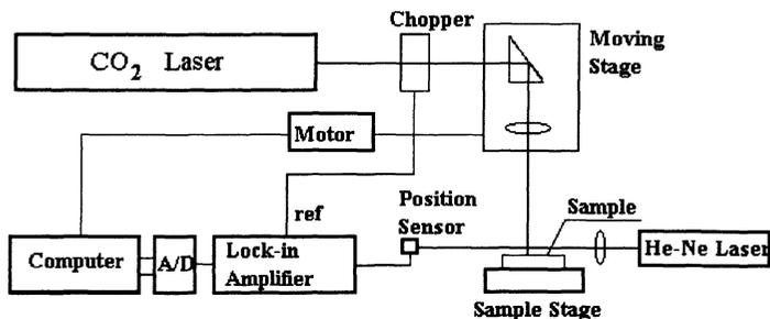
Figure 2. Experimental arrangement of 'Mirage effect' (OBD).
