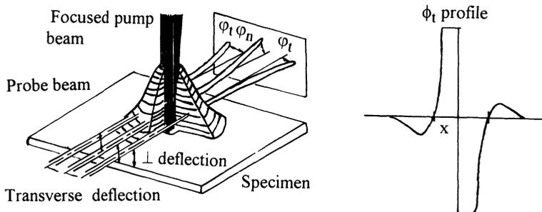
Figure 1. Schematic drawing of 'Mirage effect' (OBD method).
