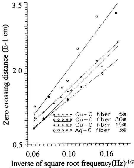
Figure 3. Zero crossing distances  $x$  versus inverse square root frequencies  $(\sqrt{f})^{-1/2}$  for Ag-Cf and Cu-Cf with fractions of fibers of 3% and 5%, 15% as well as 30% respectively.
