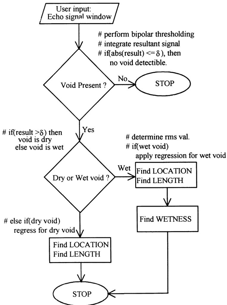
Figure 8. Flowchart for echo waveform classification.
