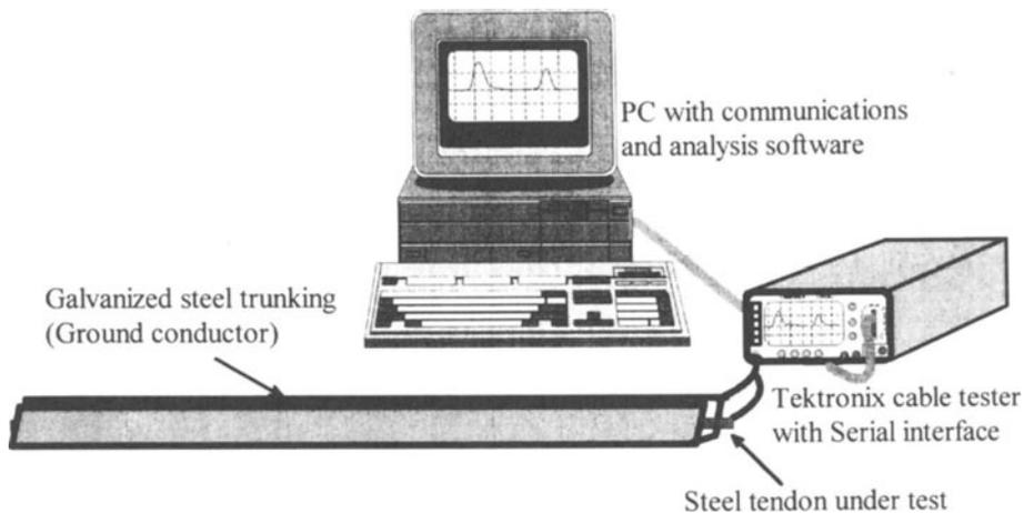
Figure 3. Equipment configuration for ETDR measurements and echo waveform classification.
