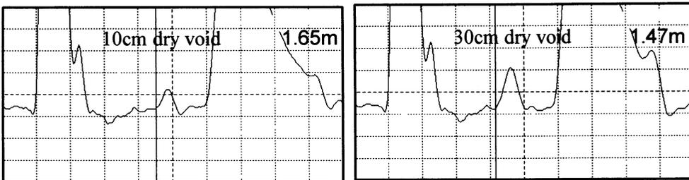
Figure 5. Annotated 1503C screen waveforms for different dry void lengths.
