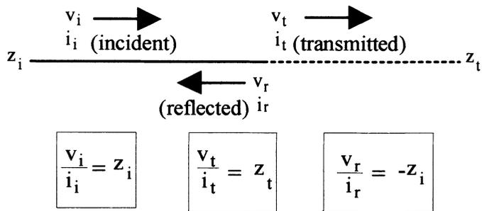
Figure 2. Wave reflection in a transmission line.
