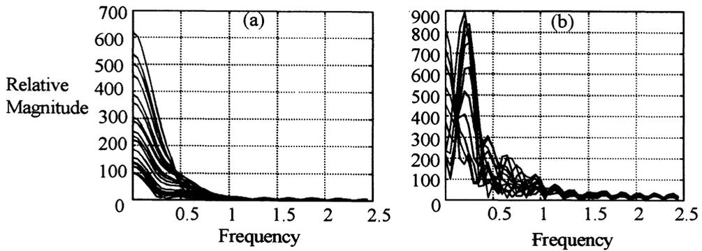
Figure 7. Fourier magnitude plots for the detection of (a) wet sections and (b) dry voids.
