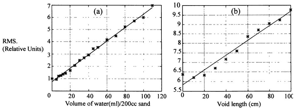
Figure 6. Echo RMS plots for the detection of (a) wet sections and (b) dry voids.
