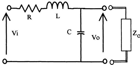
Figure 1. Lumped parameter equivalent circuit of a transmission line.
