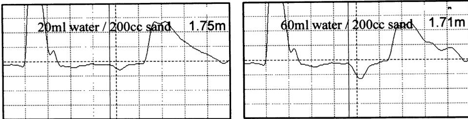
Figure 4. Annotated 1503C screen waveforms for different degrees of wetness at 1.75m.
