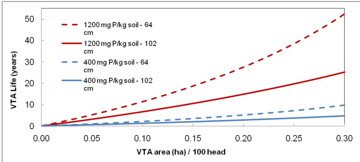
**Figure9.** The potential life expectancy range for VTAs in Iowa using a maximum and minimum phosphorus sorption capacity of 400 and 1200 mg P/kg soil and varying the vegetation uptake and average annual rainfall.
