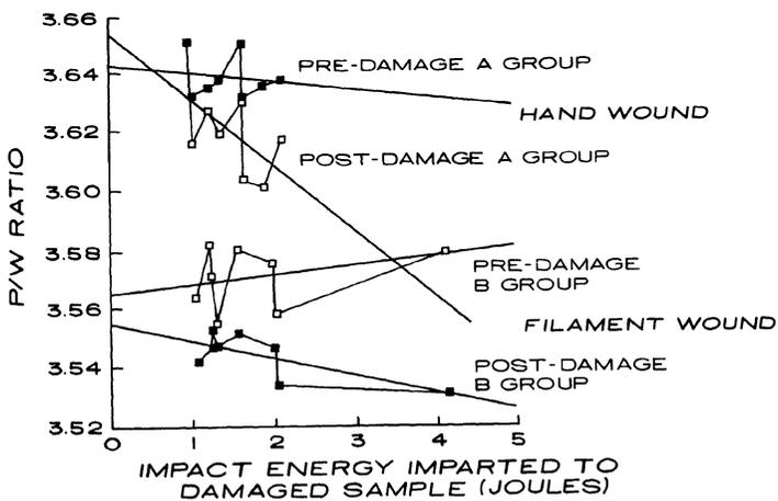
Figure 4. (P/W) ratio versus absorbed impact energy.
