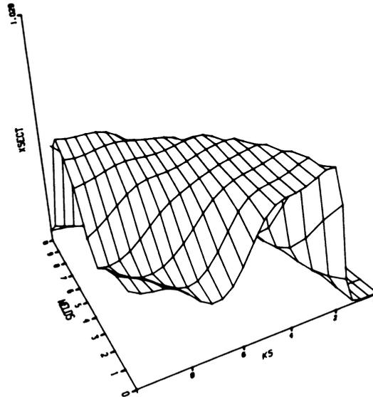
Fig. 7 SV intensity downward from partially closing crack, for incident Rayleigh wave. P scattering in this direction is negligible.
