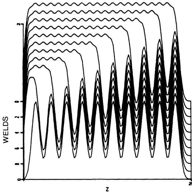
Fig. 3 Crack signatures (defined by  $\sum_{n=1}^N v_n(r)$ ) for a sequence of cracks which are increasingly (back to front) partially closed from the tip (at the right).
