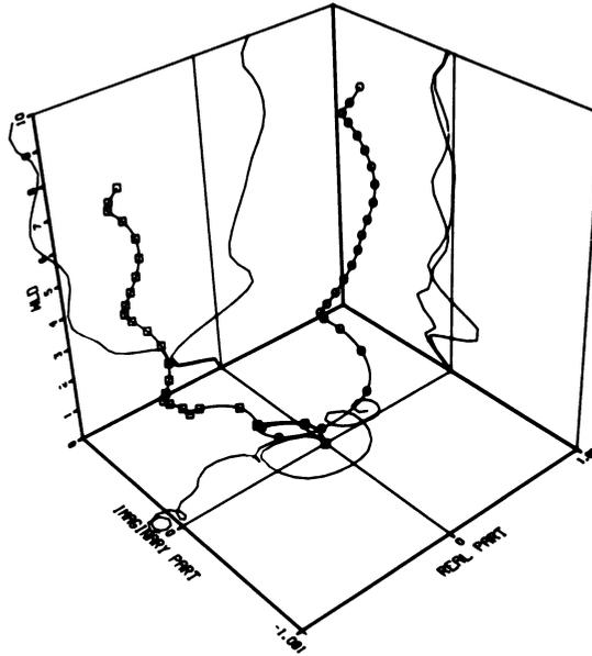
Fig. 6 Real and imaginary parts of the forward (squares) and backward (circles) Rayleigh amplitudes as functions of frequency (vertical coordinate) expressed as  $kL$ . The limits of the  $x, y$  axis are  $\pm$  (incident amplitude);<sup>s</sup> thus condition III is nearly satisfied for the transmitted amplitude.
