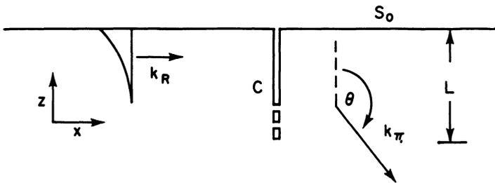
Fig. 1 Surface-breaking crack geometry. A Rayleigh wave with wave-number  $k_R$  is incident from the left; it is reflected, transmitted, and converted into bulk waves  $k_\pi$ . The origin of the  $x$ - $z$  coordinates is the crack mouth,  $C$  is the right-hand crack surface, and  $S_0$  is the  $z = 0$  plane. Overall crack length is  $L$ .
