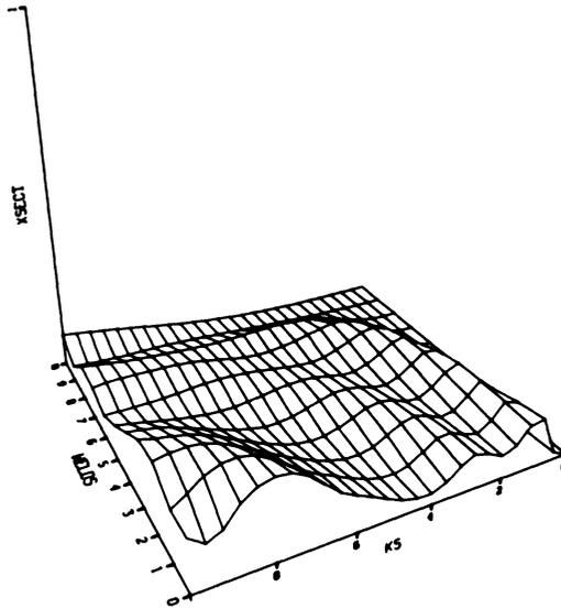
Fig. 4 Backscattered Rayleigh intensity (Rayleigh incidence) for the crack illustrated in Fig. 3. Closure increases front to back. Frequency increases from right ( $k_s L = 0$ ) to left ( $k_s L = 10$ ).
