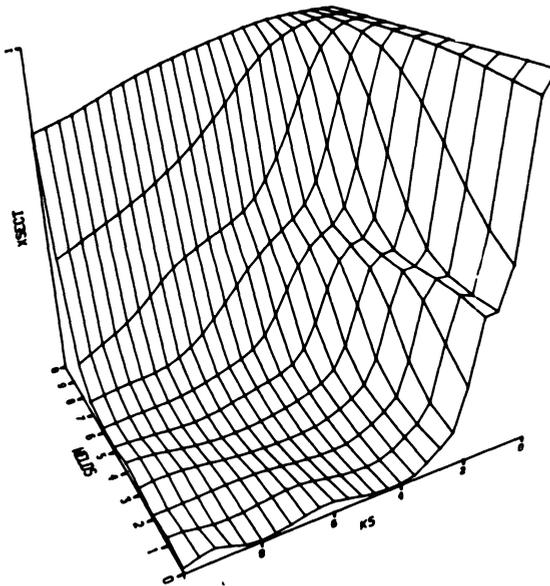
Fig. 5 Forward Rayleigh intensity for partly closing crack. The crack which is completely partially closed (10 welds) becomes nearly transparent to Rayleigh waves.
