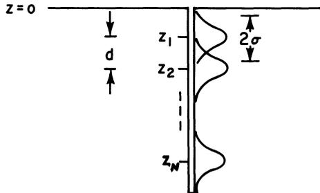
Fig. 2 The localized functions  $v_n(r)$  in which the COD is expanded are gaussians of width  $2\sigma^n$  centered at  $z = z_1, z_2, \dots, z_N$ . The  $z$ 's are equally spaced ( $z_n - z_{n-1} = d$ ); the value of  $z_1$  determines how deeply, if at all, the crack is buried.
