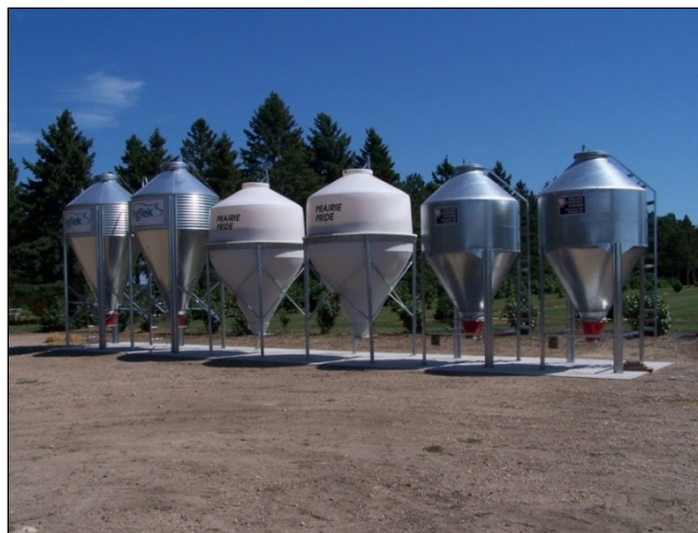
Figure 1. Bin flowability research site, West Central Research and Outreach Center, Morris, Minn. Feed bin designs were: Steel67 (two bins on left), Poly60 (two center bins), and Steel60 (two bins on right).
