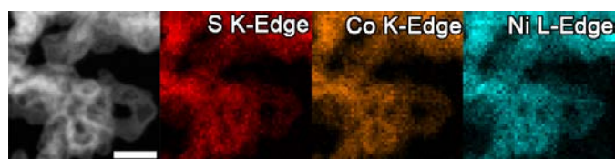
Figure 11. Registered HAADF-STEM/EDS images of the product of silylative deoxygenation of \text{NiCo}_2\text{O}_4 with \text{TMS}_2\text{S} . Scale bar = 50 nm.
