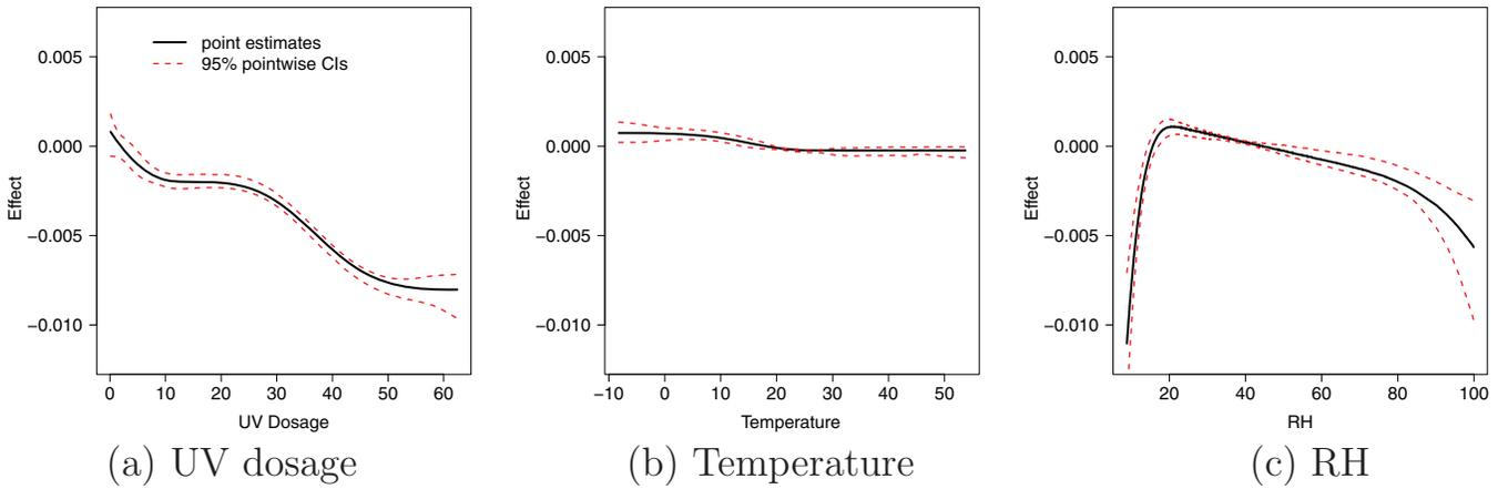
Figure 3. Estimated covariate-effect functions for UV dosage, temperature, and RH, and the corresponding approximate 95% pointwise CIs.
