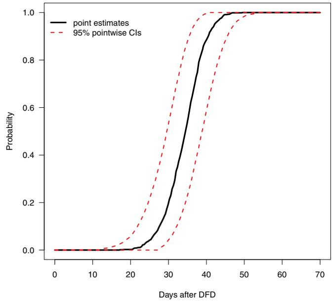
Figure 11. The estimated cdf of remaining life and 95% pointwise CIs for unit G18-10.
