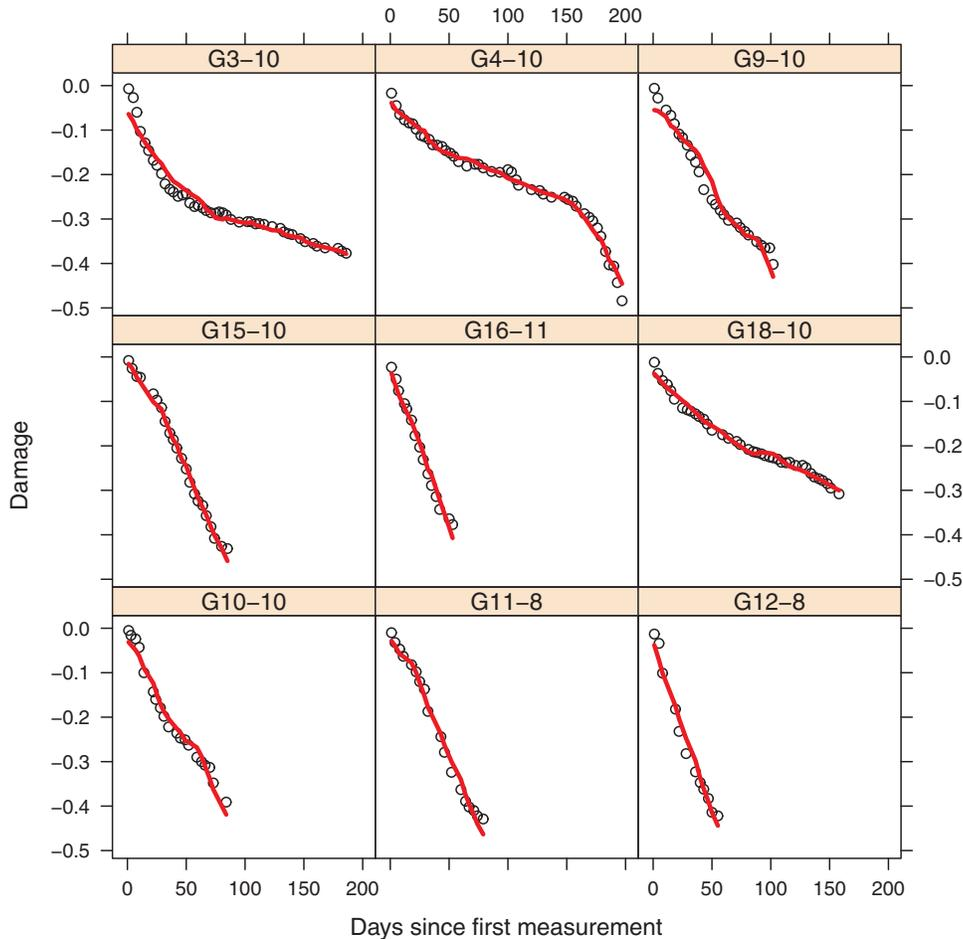
Figure 4. Plot of degradation measurements and fitted degradation path for the nine representative specimens shown in Figure 1.
