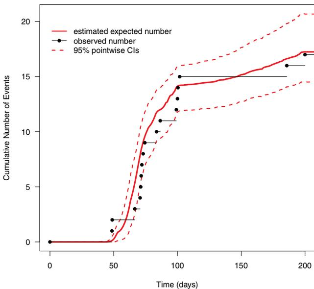
Figure 10. Estimated expected number of failures and corresponding 95% pointwise CIs versus the observed number of failures as a function of time for the 36 specimens in the outdoor weathering data, conditional on the covariate history.
