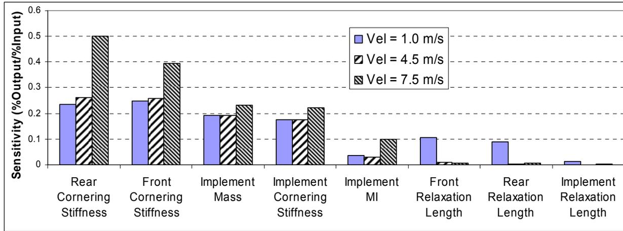
**Fig. 6: Local sensitivities at a sample point in the parameter space with respect to various system parameters at 1.0 m/s, 4.5 m/s and 7.5 m/s forward velocities.**
