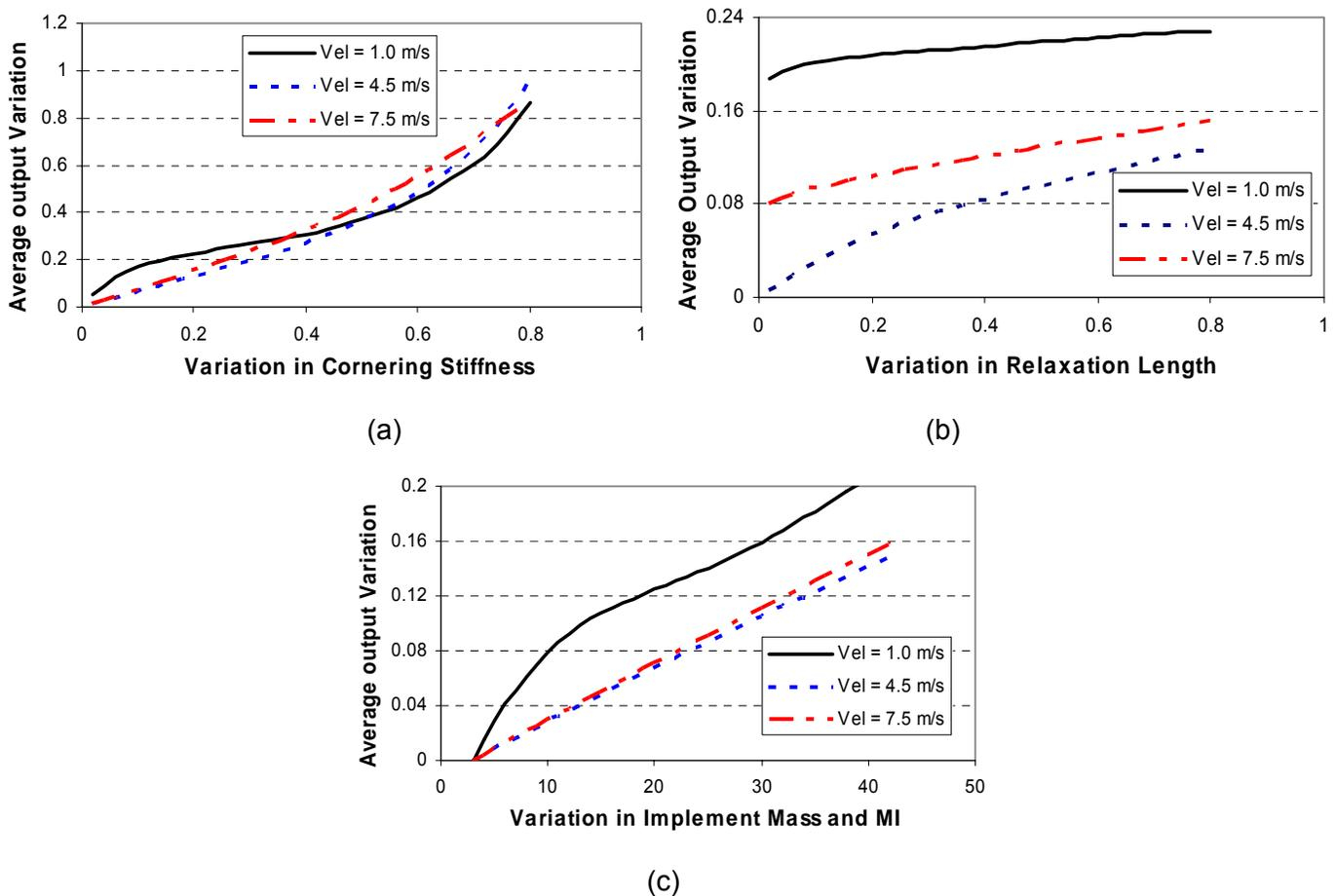
**Fig. 8:** The relationship between average variation over the six output variables of the system and the variation in a) cornering stiffness parameters, b) tire relaxation length parameters, and c) implement inertial parameters (mass and MI). The variations were calculated at 1.0 m/s, 4.5 m/s and 7.5 m/s forward velocities.
