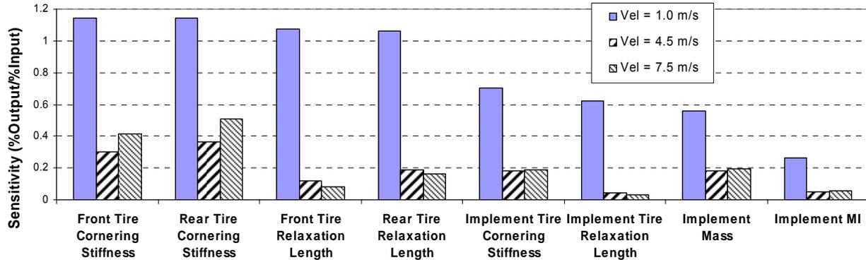
**Fig. 5: Local sensitivities at nominal point in the parameter space with respect to various system parameters at 1.0 m/s, 4.5 m/s and 7.5 m/s forward velocities.**
