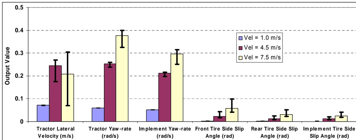
**Fig. 7: Changes in state/output variables for a 50% change in cornering stiffness parameters at 1.0 m/s, 4.5 m/s and 7.5 m/s. The solid bars represented the values of the output variables for the nominal parameters and the vertical lines represented the values of the output variables when the cornering stiffness parameters were increased and decreased by 50% of the nominal values.**
