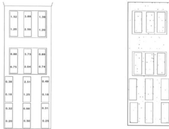
Figure 3a. Comparison of calculated and experimental amount of porosity. (top: exp. bottom: calculated); 3b. Distribution of porosity from calculation.
