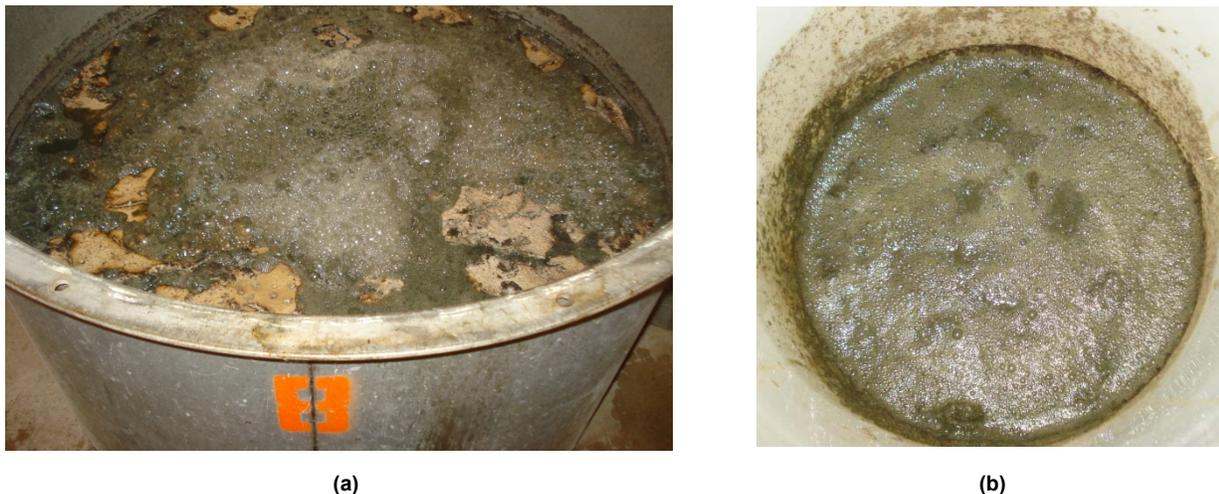
**Figure 1. (a) Foam accumulation after aeration on the surface of a tank used to collect manure in the diet studies and (b) a picture of the surface of a sample from the bucket additive study after mixing gently.**
