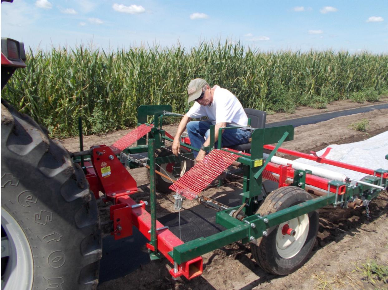
Figure 1. Tunnel layer inserting wire hoops and establishing row cover over hoops.
