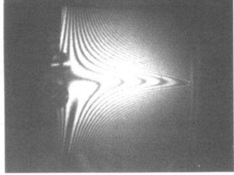
Figure 3. Fringe patterns showing first bending and first torsional modal geometries.
