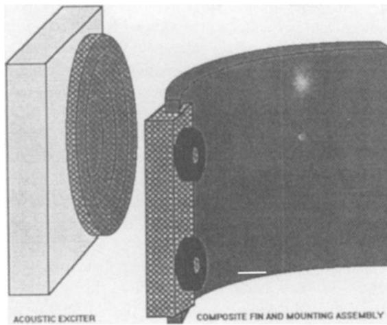
Figure 2. Graphite-epoxy composite structure assembly configuration.
