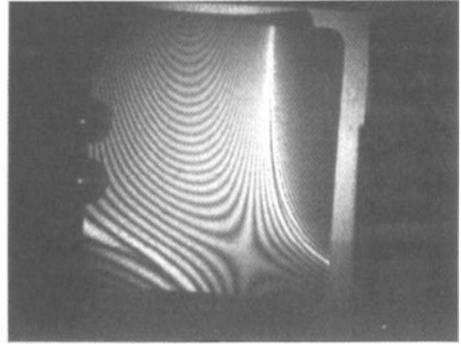
Figure 4. Holograms of bending/torsional conjugate modes.
