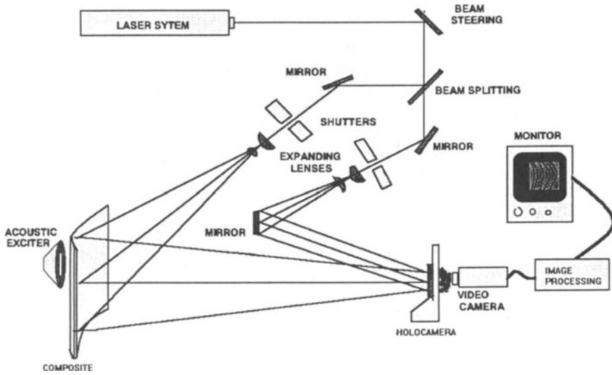
Figure 1. Holographic interferometry system.
