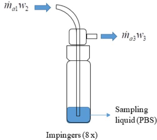
**Figure 3.** Mass balance of water vapor in the impinger to trap aerosolized virus into sampling liquid. A visual demonstration supplements Eqn. [7]; the water vapor content arriving in the impinger plus the water vapor content absorbed from the sampling liquid is equal to the water vapor content exiting the impinger. (Published as Figure 3 in Li et al., 2021a under CC BY license).
