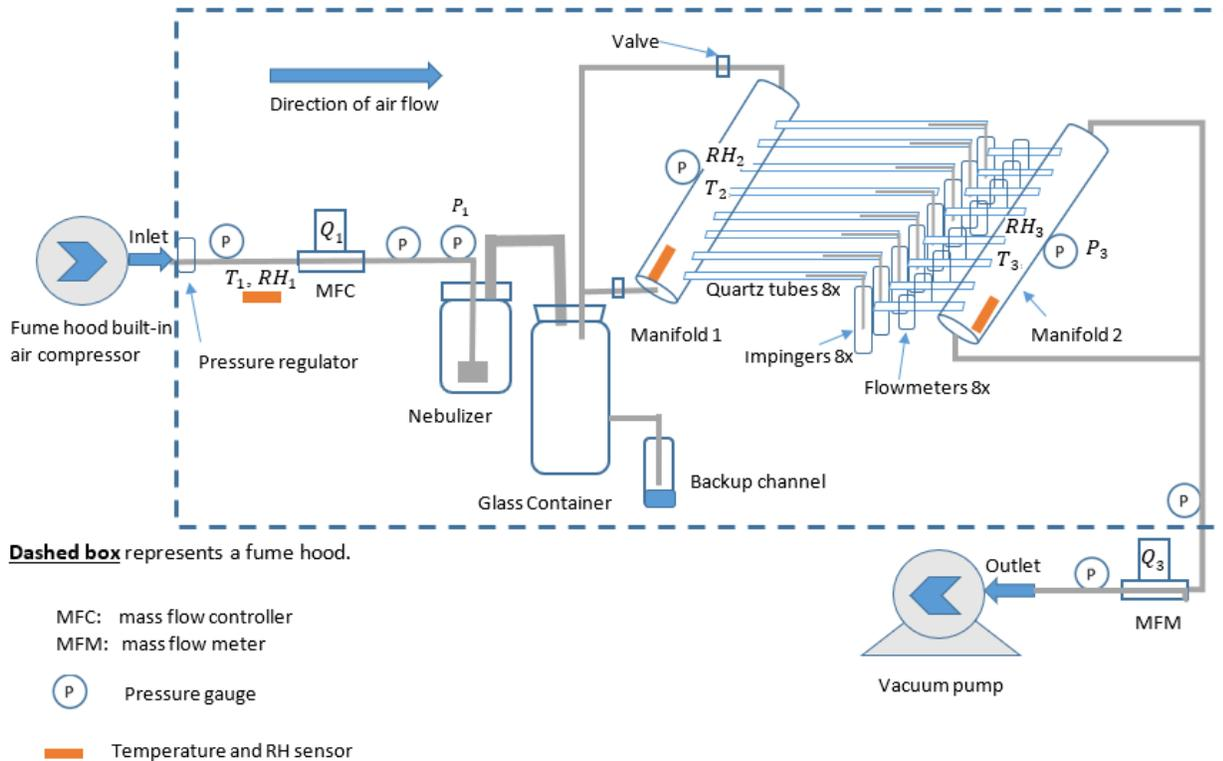
**Figure 1.** Experimental setup for generation and collection of airborne PRRSV inside a fume hood. The built-in air compressor in the fume hood was responsible for pressurizing air flowing into the system, and the right-side pump was vacuuming exhaust air coming out of the system. MFC = mass flow controller; MFM = mass flow meter. (Published as Figure 1 in Li et al., 2021a under CC BY license).
