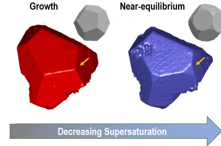
**Figure 1.** The growth and near-equilibrium shape of an icosahedral  $\text{Al}_{71}\text{Pd}_{19}\text{Mn}_{10}$  quasicrystal.
