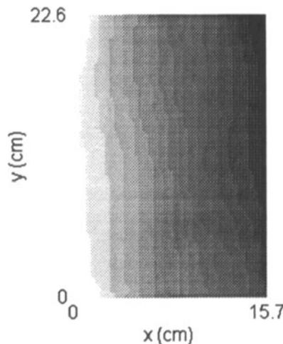
Figure 3. Image representation of the magnetic field generated by an 1m x 1m x 1mm aluminum plate with an 8 mm hole in the center, carrying 5 A current. Each level of gray corresponds to a different value of the detected magnetic field. The signal was detected by our SQUID system at a 9 cm standoff distance. The image has been displayed to present maximum dynamic range.
