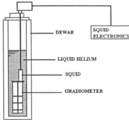
Figure 2. SQUID system consisting of the SQUID sensor, gradiometer, liquid helium dewar and electronics.
