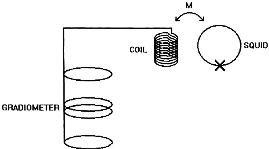
Figure 1. Schematic view of the SQUID coupled to a flux transformer consisting of a second order gradiometer and a secondary coil. The diameter of each coil is 1.5 cm and the distance between each set of coils is 4 cm.
