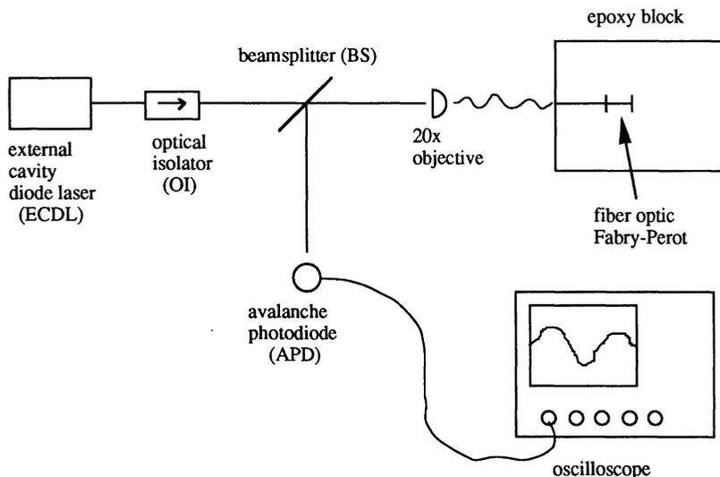
Figure 3: Schematic of experiment with local FOFP.
