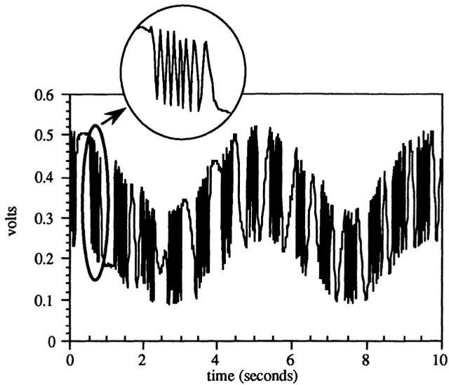
Figure 4: Reflected intensity from double cavity as frequency is shifted.
