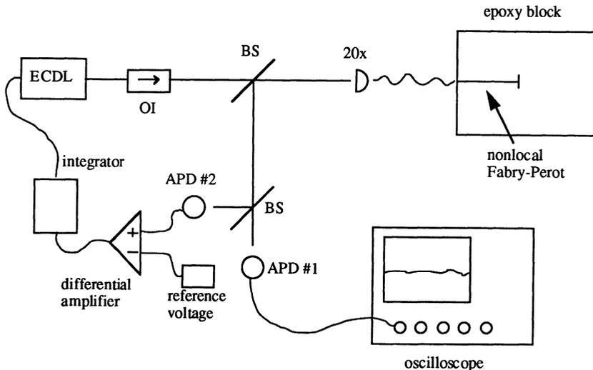
Figure 5: Schematic of experiment for stabilization of nonlocal FOFP.
