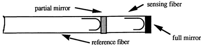
Figure 1: Schematic of FOFP.
