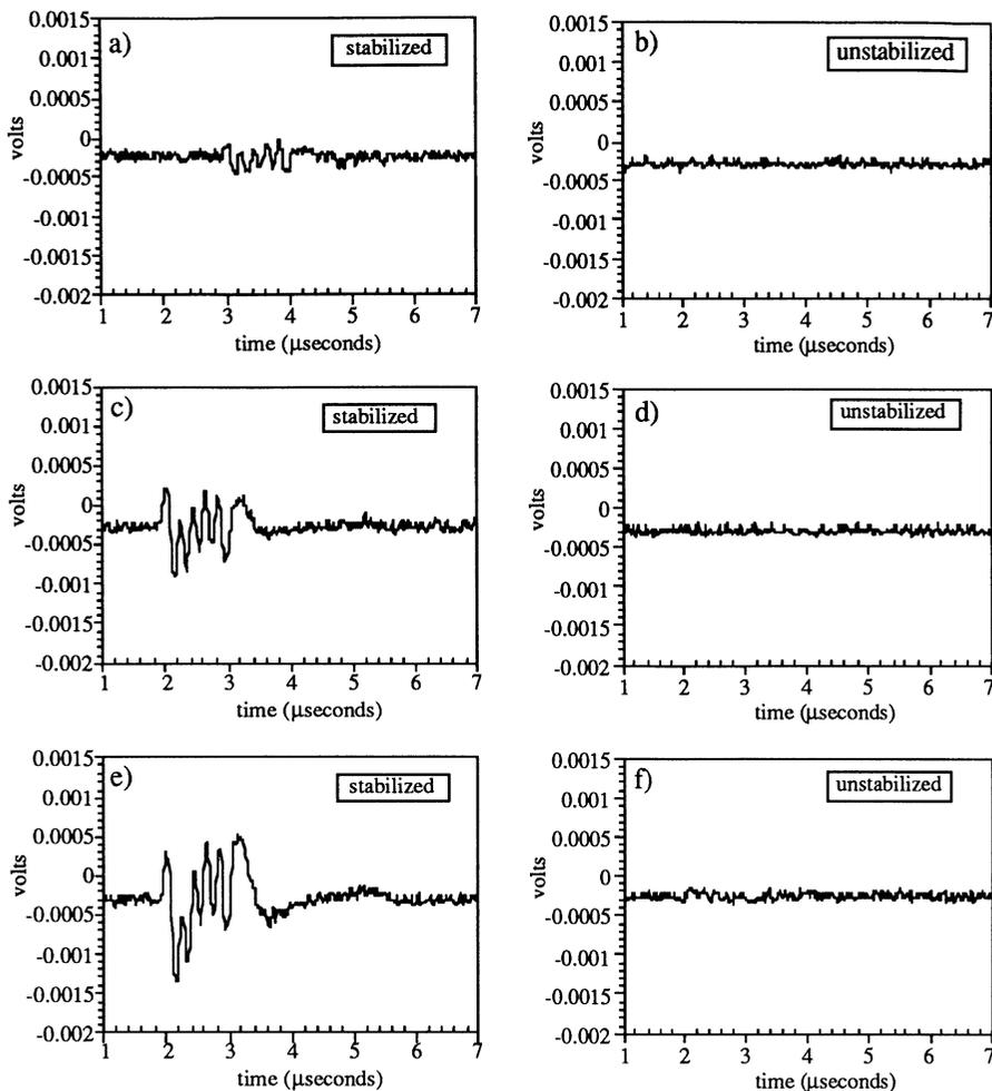
Figure 9: 5MHz toneburst detected with nonlocal FOFP stabilized and unstabilized.
