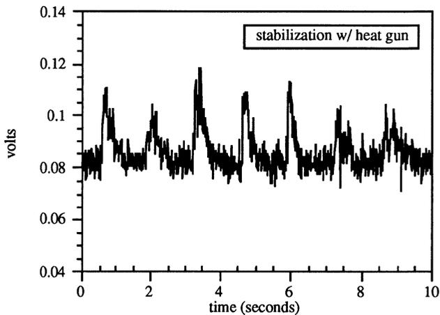
Figure 8: Reflected intensity from stabilized nonlocal FOFP with heat gun induced drift.
