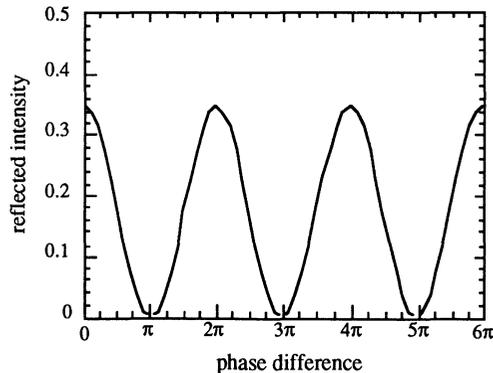
Figure 2: Normalized reflected intensity vs. phase shift.
