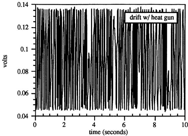
Figure 7: Reflected intensity from unstabilized nonlocal FOFP with heat gun induced drift.
