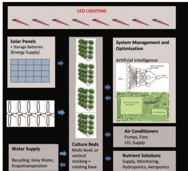
Figure 2. Layout for an indoor vertical farm. (Photo courtesy of Benke & Tomkins, 2017)
