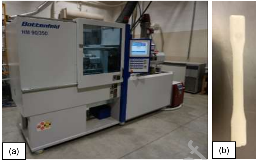
Fig. 1. (a) Battenfeld HM90/350 90-ton horizontal injection molder and an (b) ASTM Type I Dog Bone
