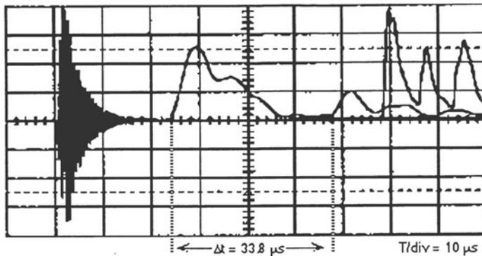
Figure 4. Optical fiber outputs after 1000 averages for the aluminum bar with BA-F113SC epoxy.
