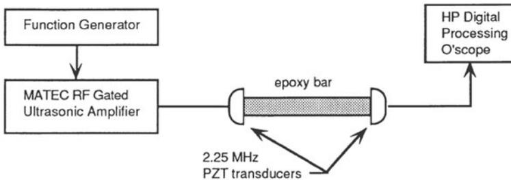
Figure 2. Epoxy characterization schematic
