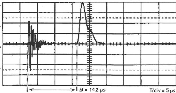
Figure 3. Acoustic transducer plot for epoxy bar characterization.
