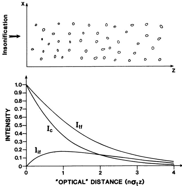
Fig. 1. Approximate behavior of the coherent intensity  $I_c$ , the forward propagating incoherent intensity  $I_{if}$ , and the total forward propagating intensity  $I_{tf}$  for an absorption free medium in the case of isotropic scattering.
