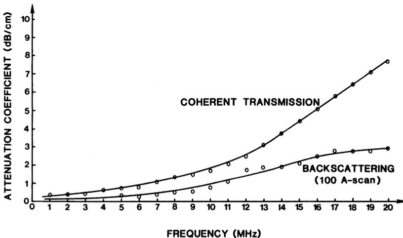
Fig. 4. Grain scattering induced attenuation in polycrystalline Copper.
