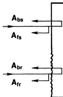
Fig. 2. Schematic diagram of the surface roughness induced attenuation measurement.
