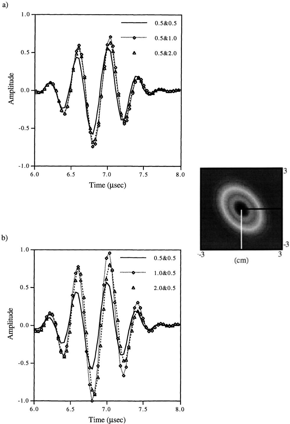
Figure 5. Response from the crack for  $30^\circ$  azimuthal angle, a) variation with crack depth in centimeters , b) variation with crack length in centimeters.
