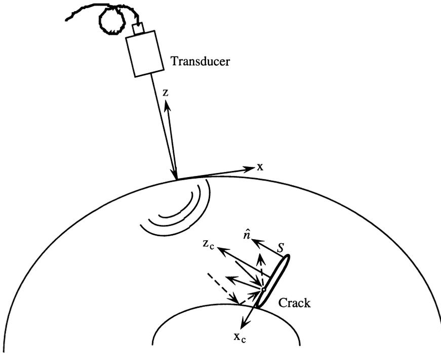
Figure 1. Geometrical configuration of the interfaces, the crack and the coordinate systems.
