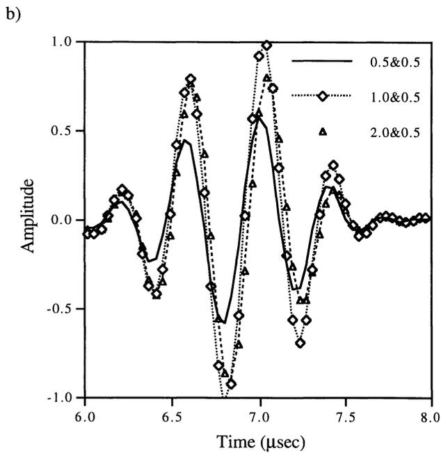
Figure 6. Response from the crack for  $90^\circ$  azimuthal angle, a) variation with crack depth in centimeters, b) variation with crack length in centimeters.
