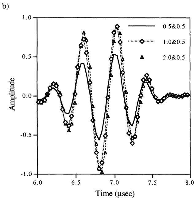
Figure 4. Response from the crack for  $0^\circ$  azimuthal angle, a) variation with crack depth in centimeters, b) variation with crack length in centimeters.
