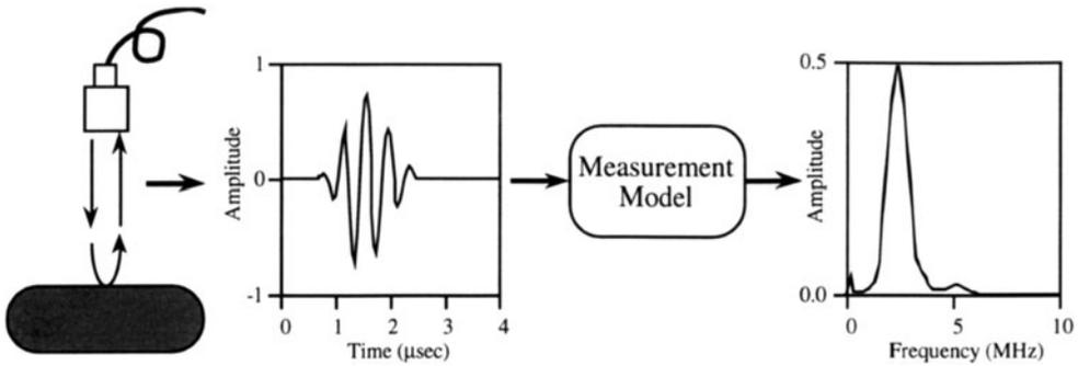
Figure 2. Schematic drawing of finding frequency spectrum of signal emitted by a transducer.
