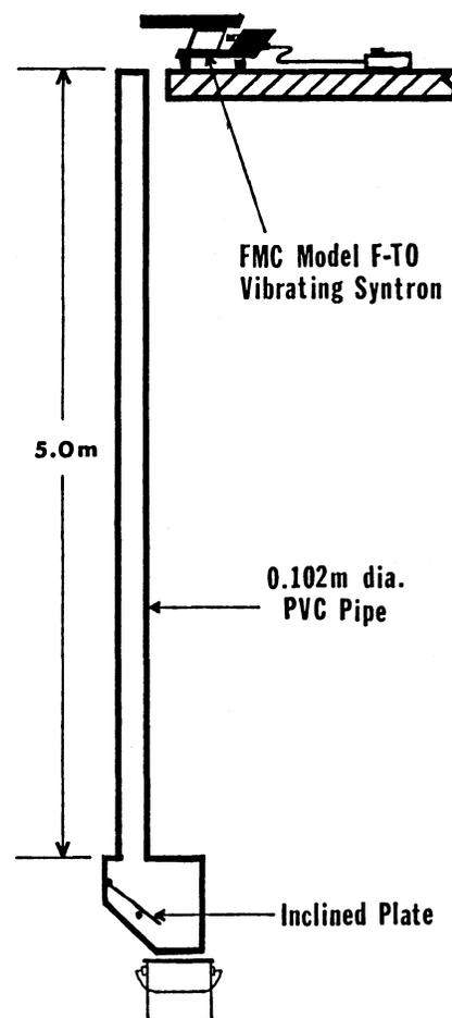
Fig. 3—Set-up used to determine breakage susceptibility of samples.
