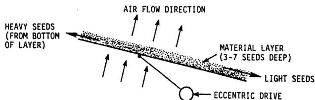
Fig. 1—Typical gravity separator cross section.
