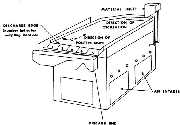
Fig. 2—Perspective view of Oliver model 50 gravity separator used for this study (drawing adapted from photo provided by Oliver Mfg. Co., Rocky Ford, CO).
