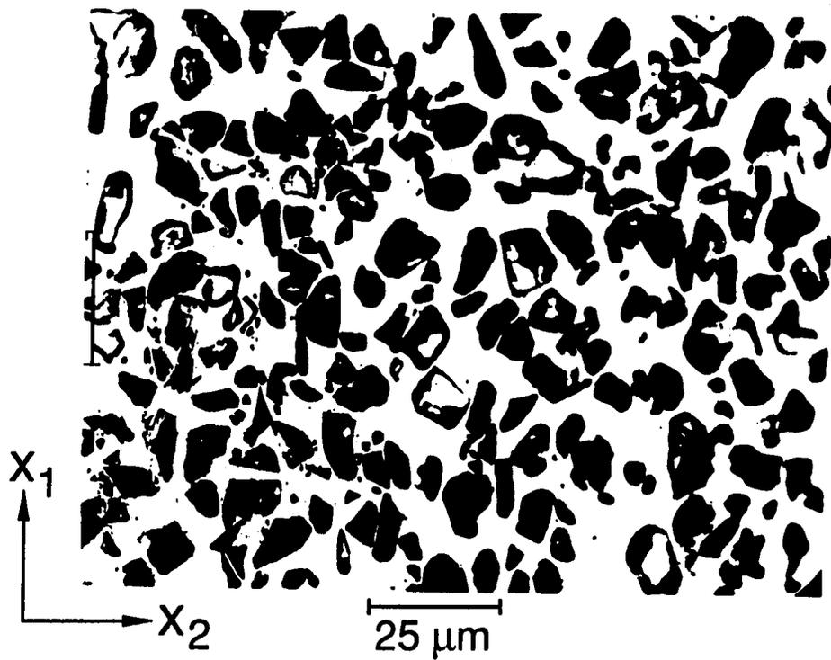
Figure 5.1: Photomicrograph taken on the  $x_1$ - $x_2$  plane of 30% SiC<sub>p</sub>/7091 Al (PE-2665)
