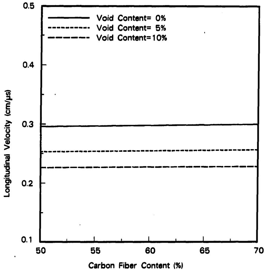
Figure 2.4: Effect of fiber content on ultrasonic velocity (carbon fiber composite)
