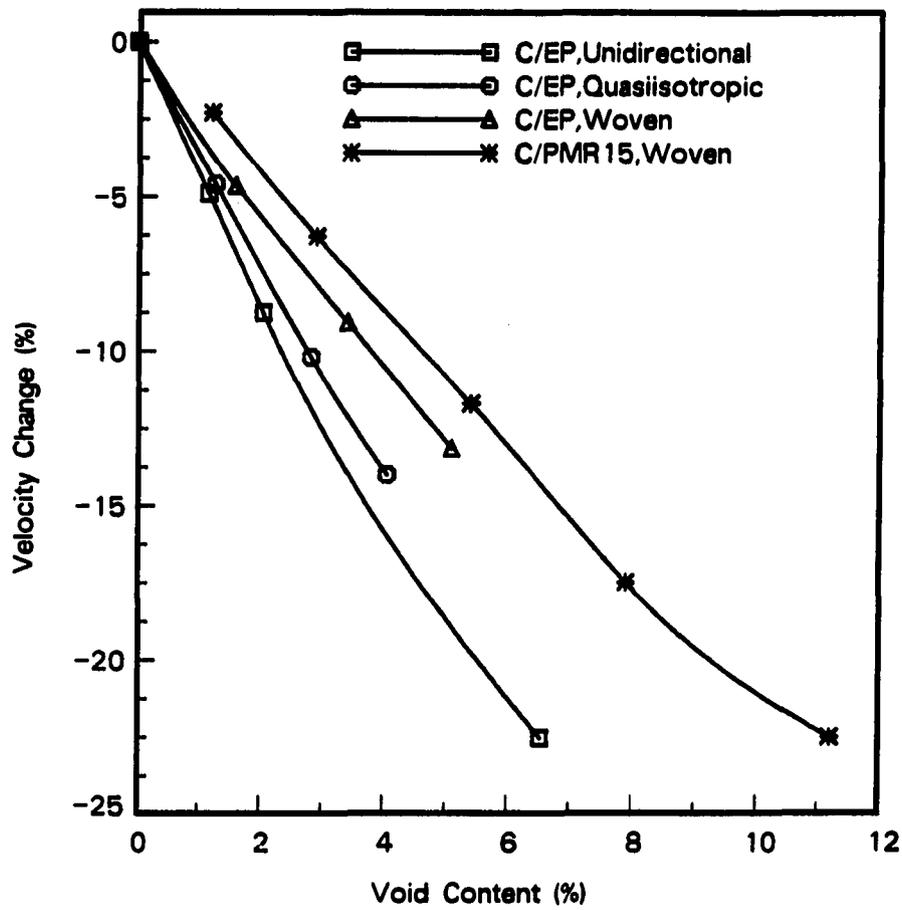
Figure 4.7: Velocity change versus void content at 2 MHz
