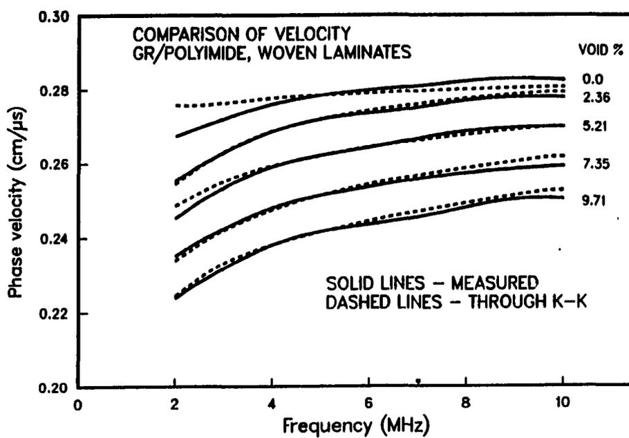
Figure 5.1: Comparison of measured velocity in carbon/polyimide composites with calculated velocity using Kramers-Kronig relation
