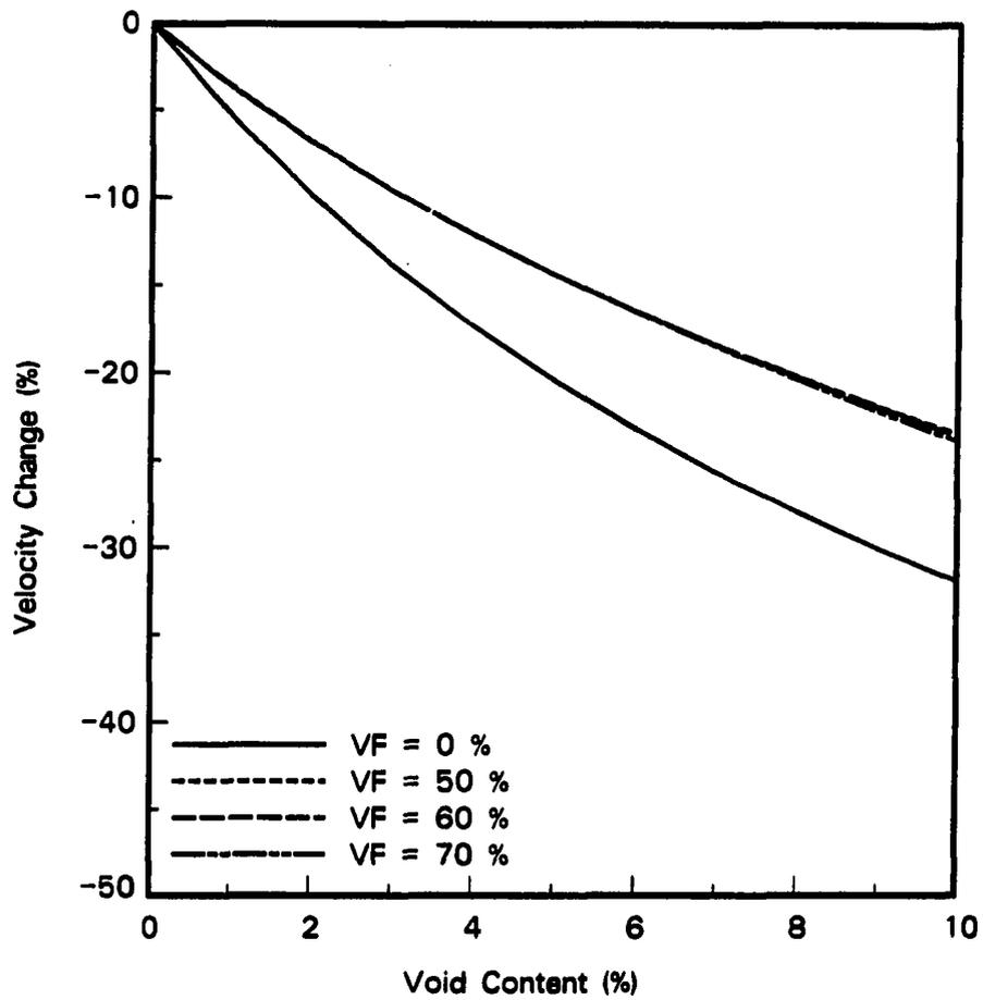
Figure 2.2: Effect of void content on ultrasonic velocity (carbon fiber composite)
