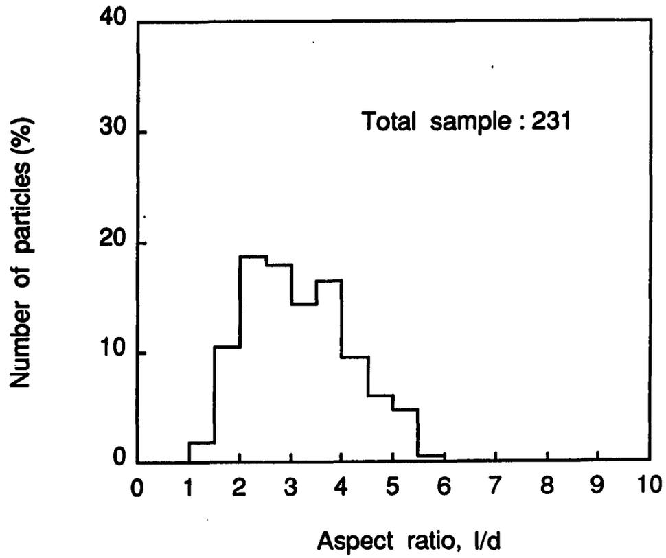
Figure 5.6: SiC<sub>p</sub> aspect ratio distribution on the  $x_2$ - $x_3$  plane of 30% SiC<sub>p</sub>/7091 Al sample (PE-2665)
