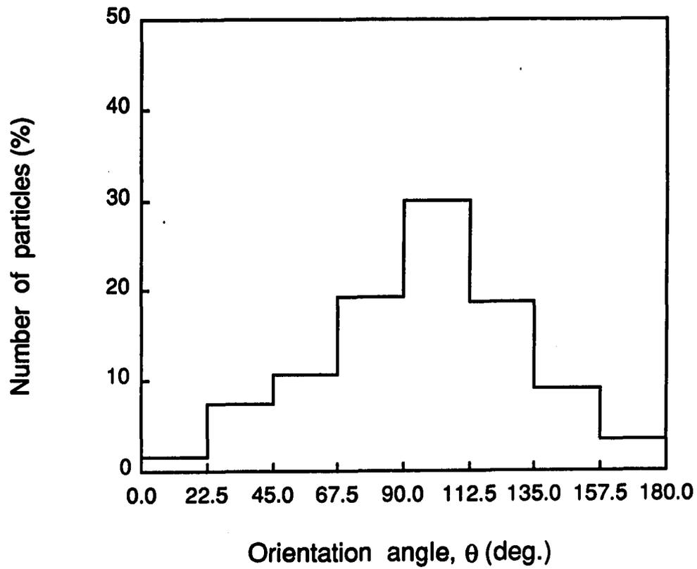
Figure 5.8: SiC<sub>p</sub> orientation distribution on the  $x_1$ - $x_3$  plane of 30% SiC<sub>p</sub>/7091 Al sample (PE-2665)
