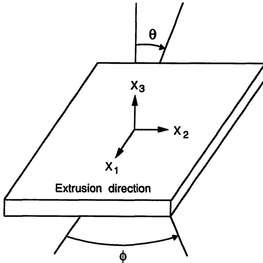
Figure 3.1: Material symmetry axes for orthotropic plate
