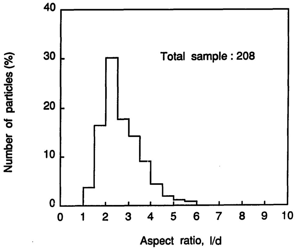
Figure 5.4: SiC<sub>p</sub> aspect ratio distribution on the  $x_1$ - $x_2$  plane of 30% SiC<sub>p</sub>/7091 Al sample (PE-2665)
