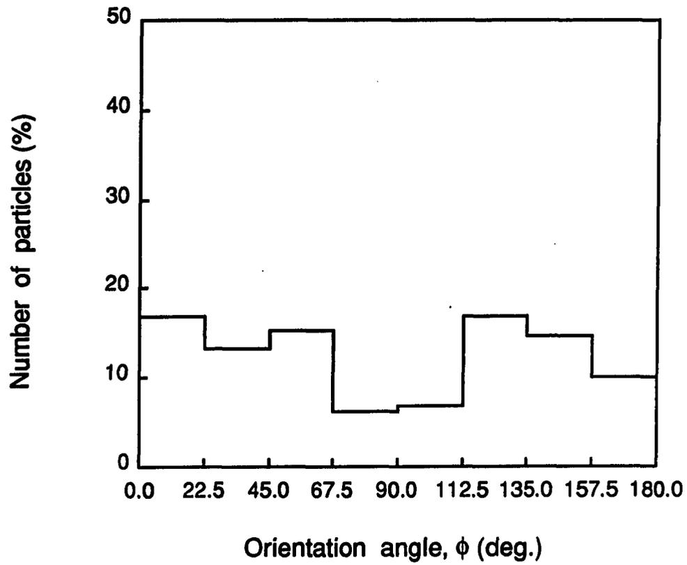
Figure 5.7:  $\text{SiC}_p$  orientation distribution on the  $x_1$ - $x_2$  plane of 30%  $\text{SiC}_p$ /7091 Al sample (PE-2665)
