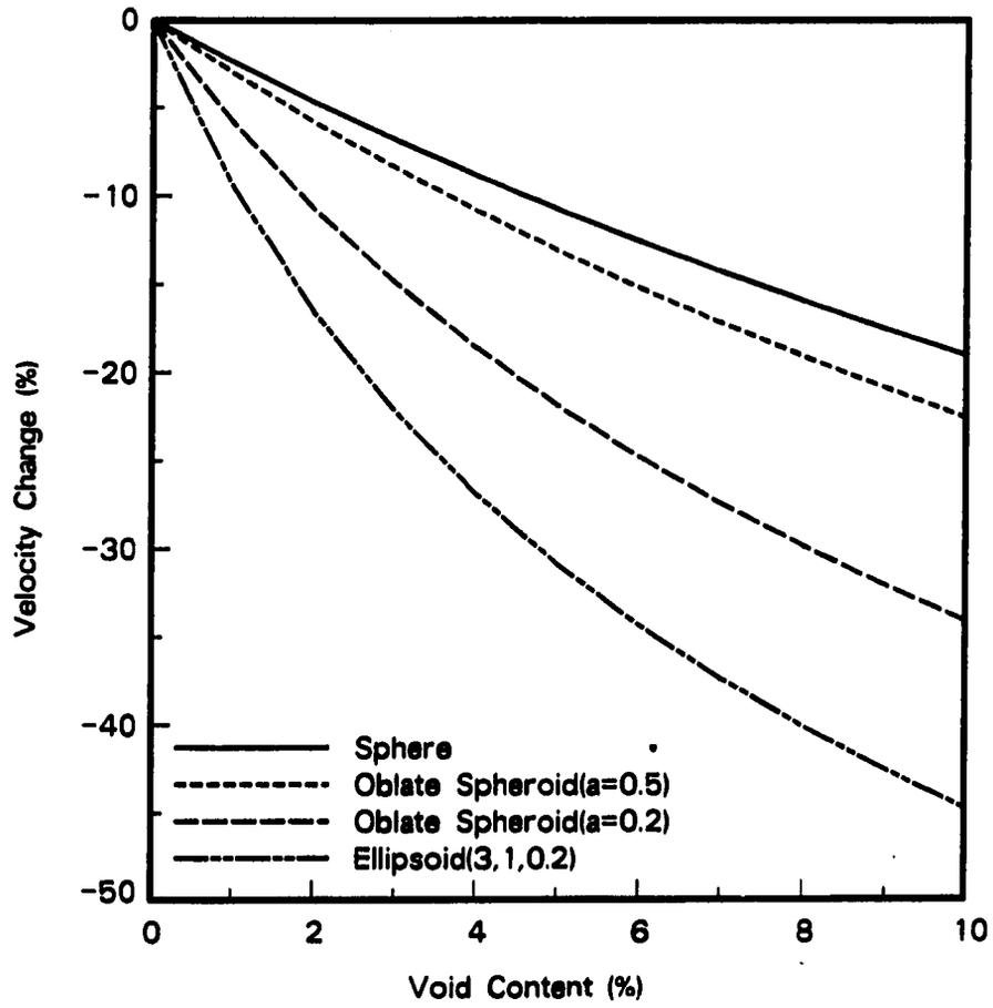
Figure 2.5: Effect of void shape on ultrasonic velocity (fiberglass fiber composite)
