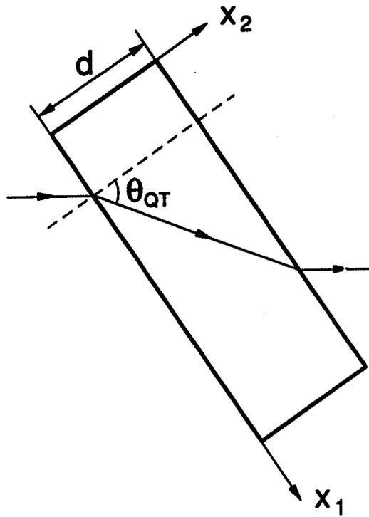
Figure 3.3: Sample orientation for measuring  $C_{66}$  and  $C_{12}$
