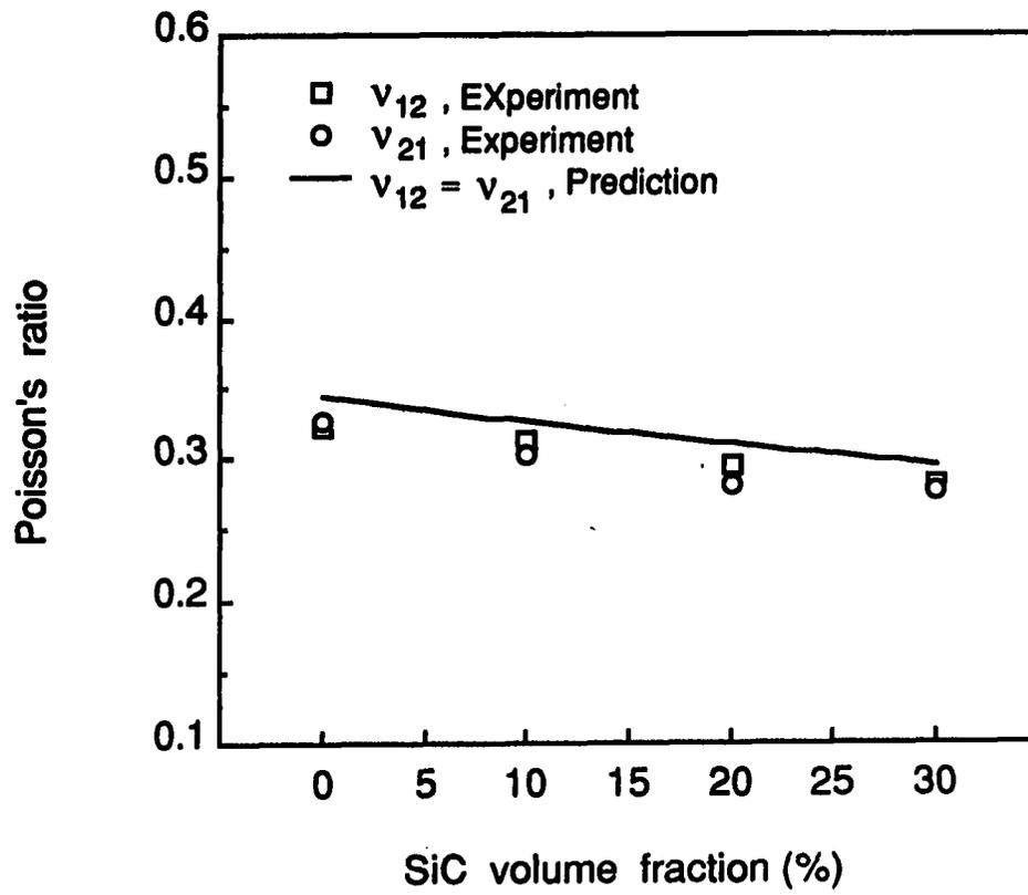
Figure 6.6: Comparison of predicted Poisson's ratios  $\nu_{12}$  and  $\nu_{21}$  with experimental results (7091 Al/SiC<sub>p</sub>)
