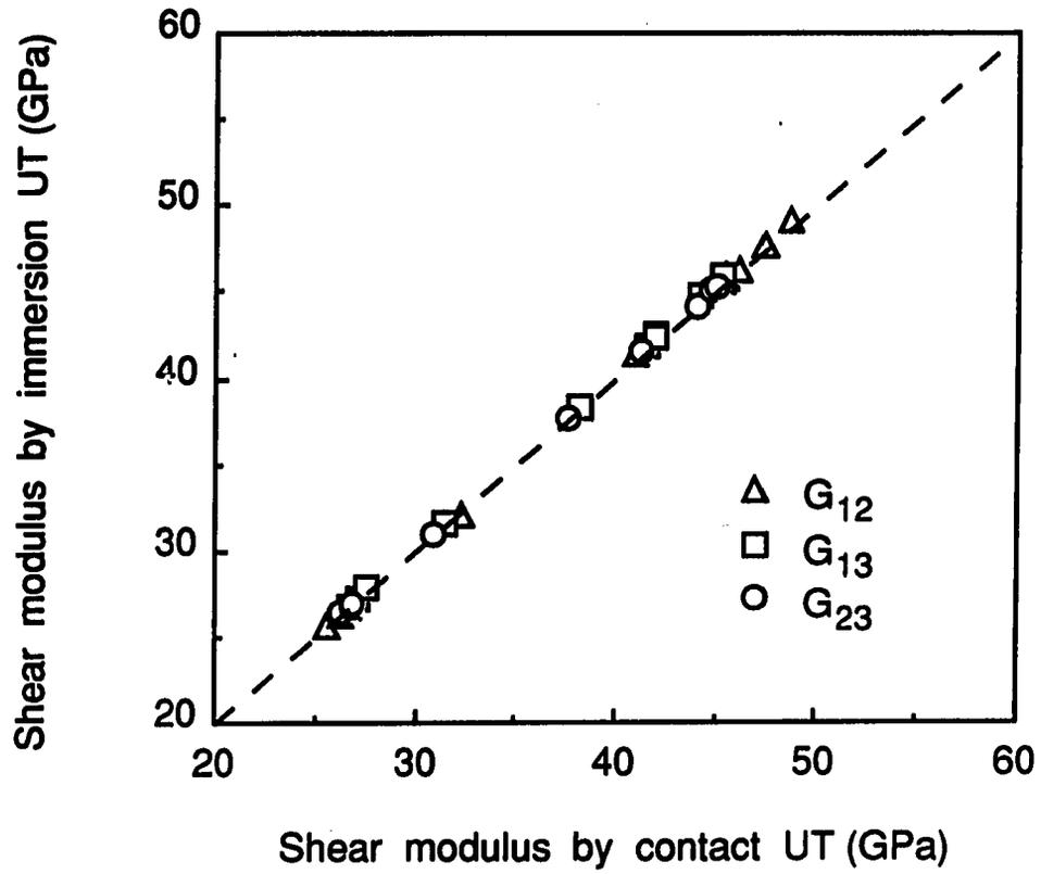
Figure 3.6: Comparison of shear moduli measured by ultrasonic immersion method with those obtained by direct contact method
