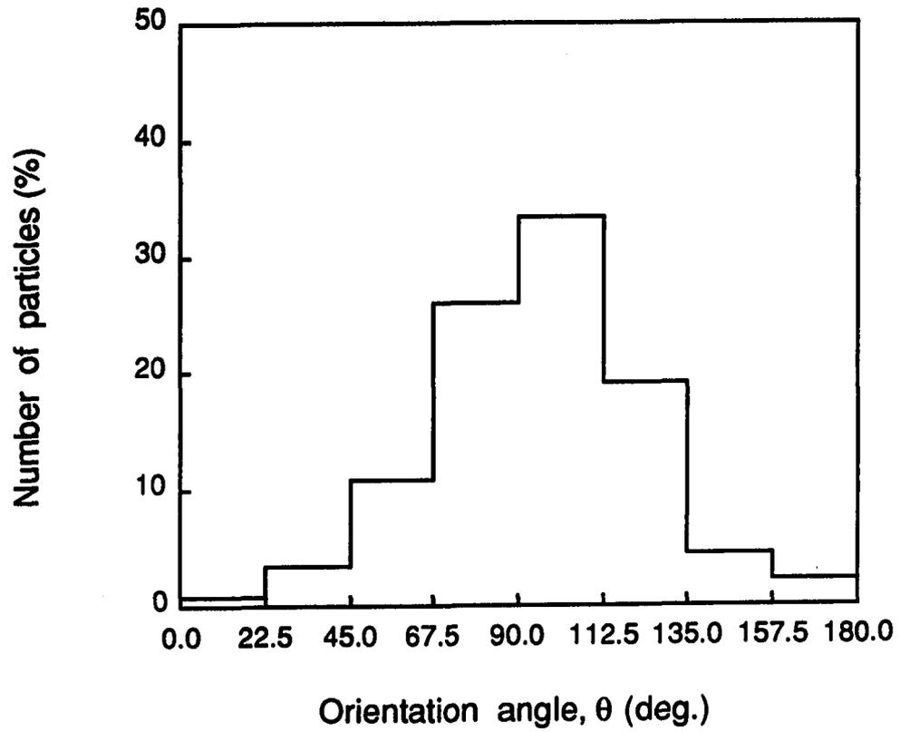
Figure 5.9: SiC<sub>p</sub> orientation distribution on the  $x_2$ - $x_3$  plane of 30% SiC<sub>p</sub>/7091 Al sample (PE-2665)
