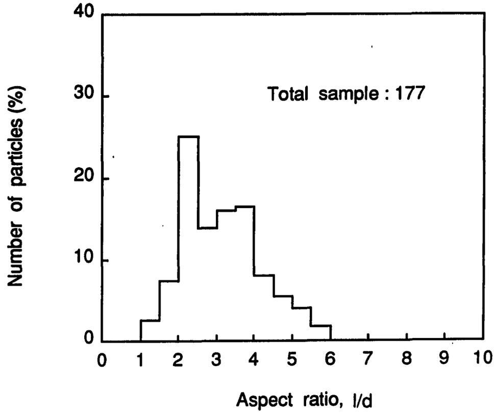
Figure 5.5: SiC<sub>p</sub> aspect ratio distribution on the  $x_1$ - $x_3$  plane of 30% SiC<sub>p</sub>/7091 Al sample (PE-2665)
