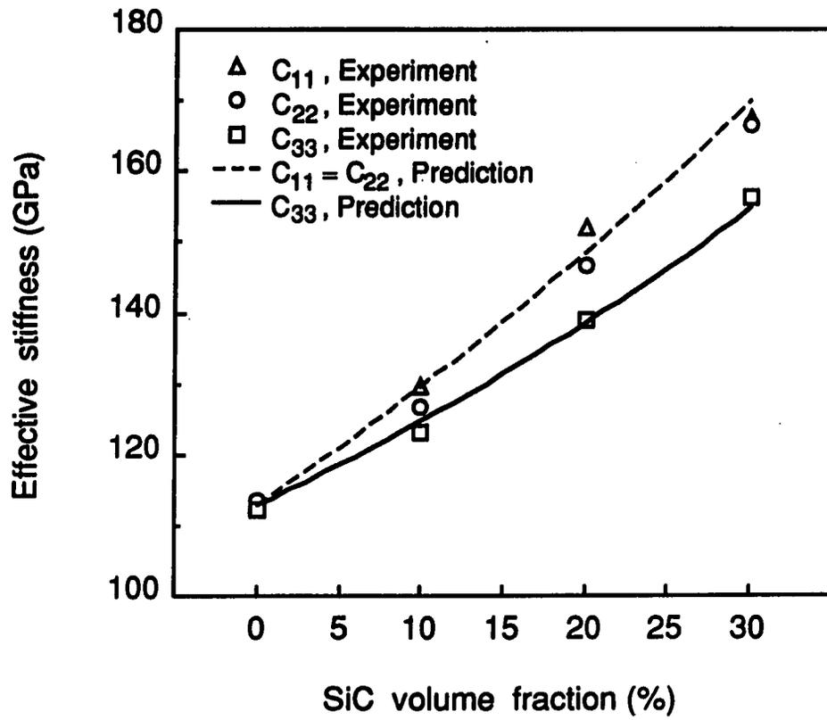
Figure 6.2: Comparison of predicted stiffnesses  $C_{11}$ ,  $C_{22}$  and  $C_{33}$  with experimental results (7091 Al/SiC<sub>p</sub>)
