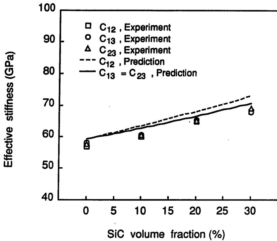
Figure 6.4: Comparison of predicted stiffnesses  $C_{12}$ ,  $C_{13}$  and  $C_{23}$  with experimental results (7091 Al/SiC<sub>p</sub>)
