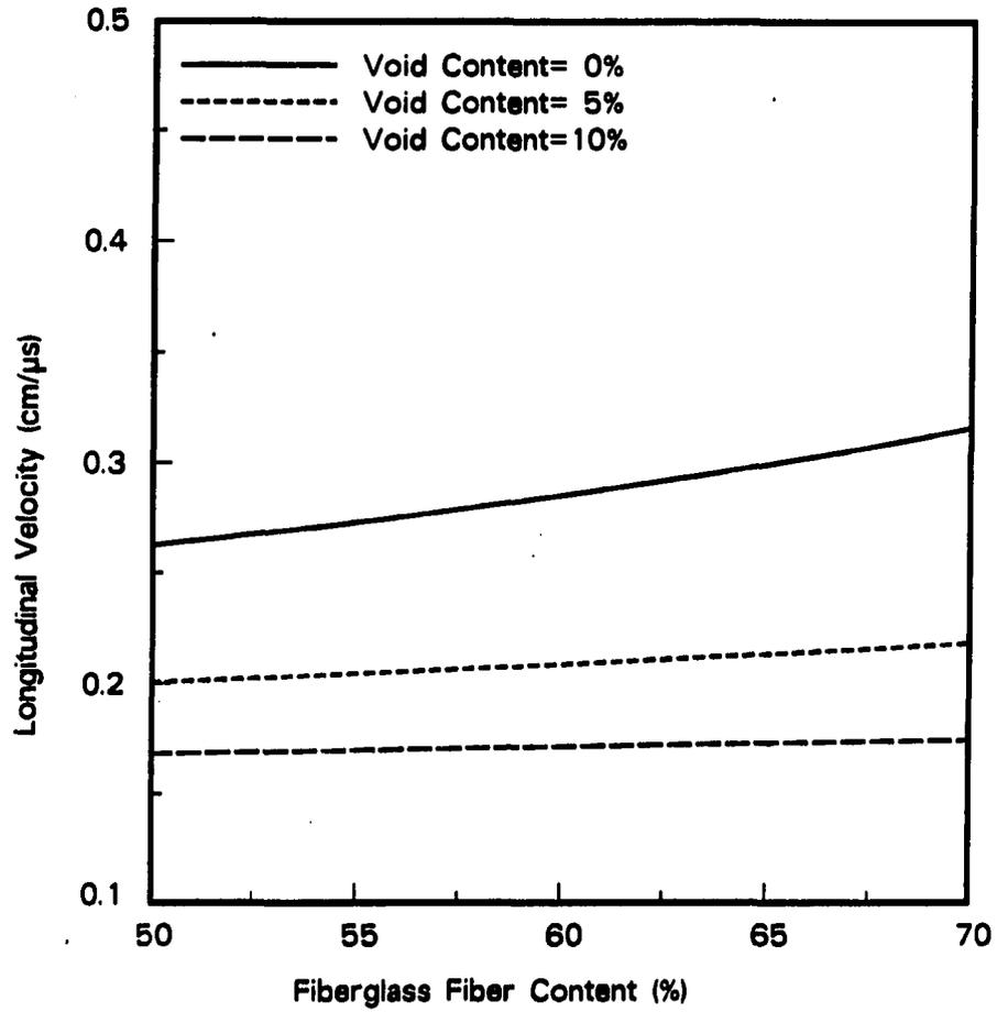
Figure 2.3: Effect of fiber content on ultrasonic velocity (fiberglass fiber composite)
