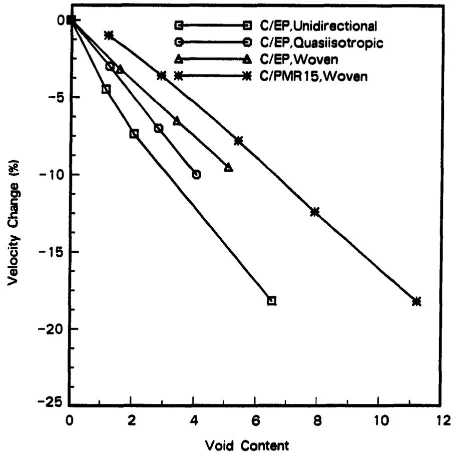
Figure 4.8: Velocity change versus void content at 5 MHz
