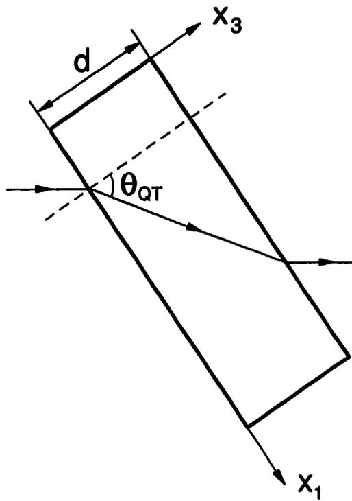
Figure 3.4: Sample orientation for measuring  $C_{55}$  and  $C_{13}$
