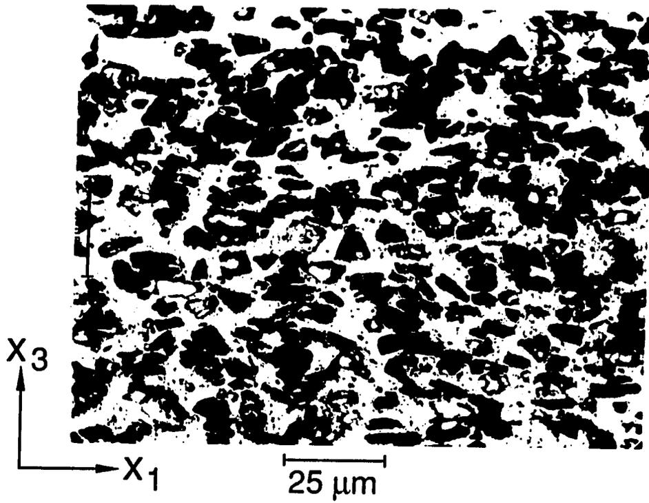
Figure 5.2: Photomicrograph taken on the  $x_1$ - $x_3$  plane of 30% SiC<sub>p</sub>/7091 Al (PE-2665)
