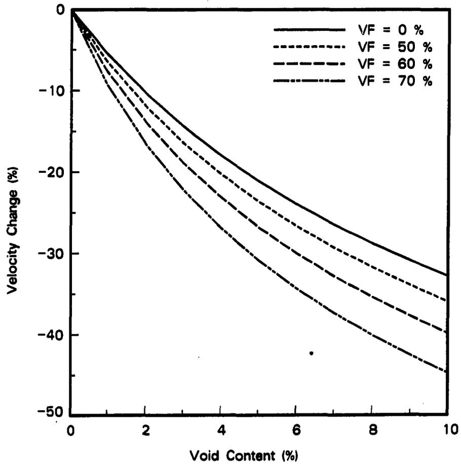
Figure 2.1: Effect of void content on ultrasonic velocity (fiberglass fiber composite)
