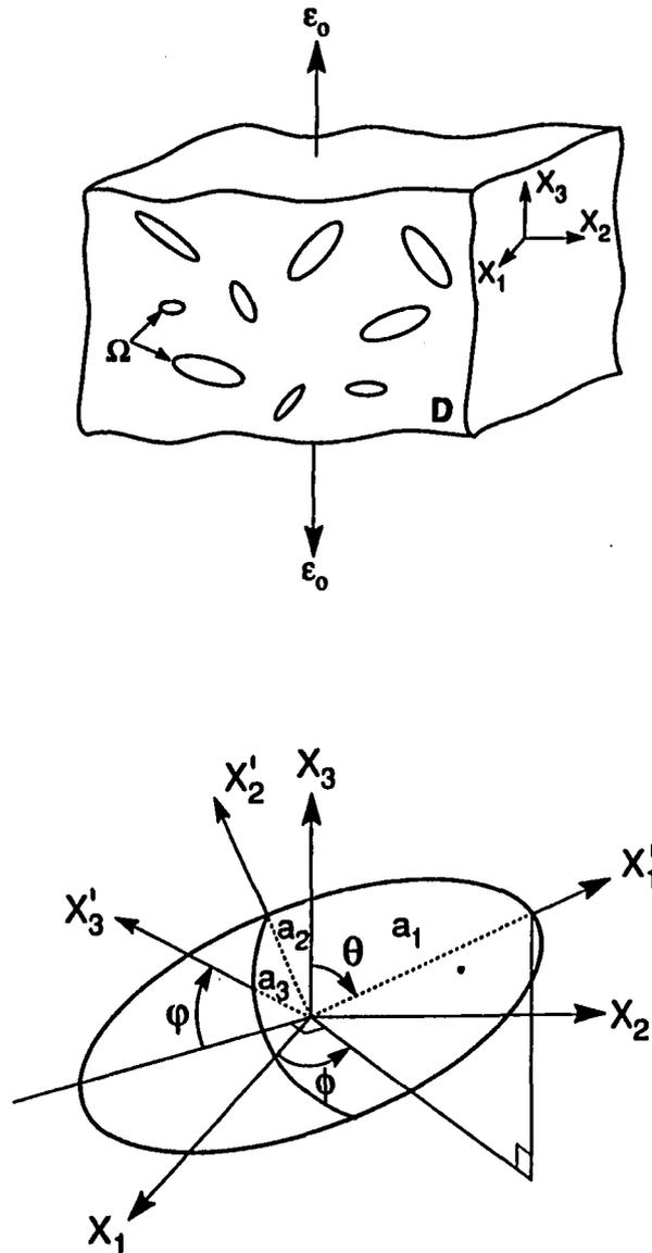
Figure 6.1: Mathematical model to predict effective stiffness of a composite containing ellipsoidal particles
