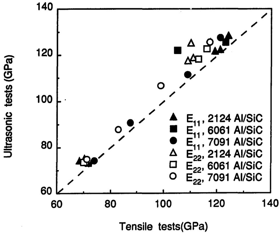
Figure 4.1: Comparison of Young's moduli measured by ultrasonic method and those obtained by tensile tests
