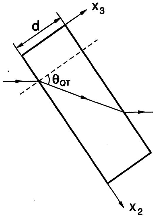
Figure 3.5: Sample orientation for measuring  $C_{44}$  and  $C_{23}$
