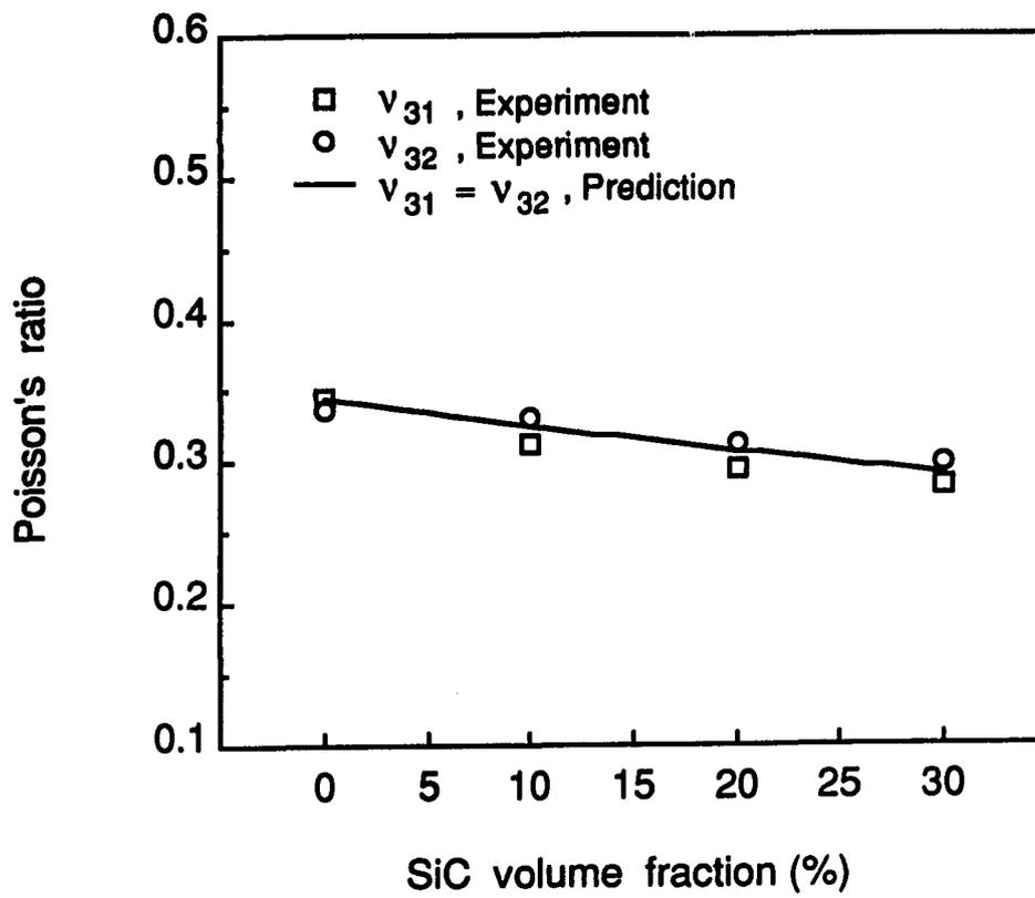
Figure 6.8: Comparison of predicted Poisson's ratios  $\nu_{31}$  and  $\nu_{32}$  with experimental results (7091 Al/SiC<sub>p</sub>)
