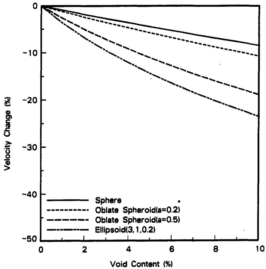
Figure 2.6: Effect of void shape on ultrasonic velocity (carbon fiber composite)
