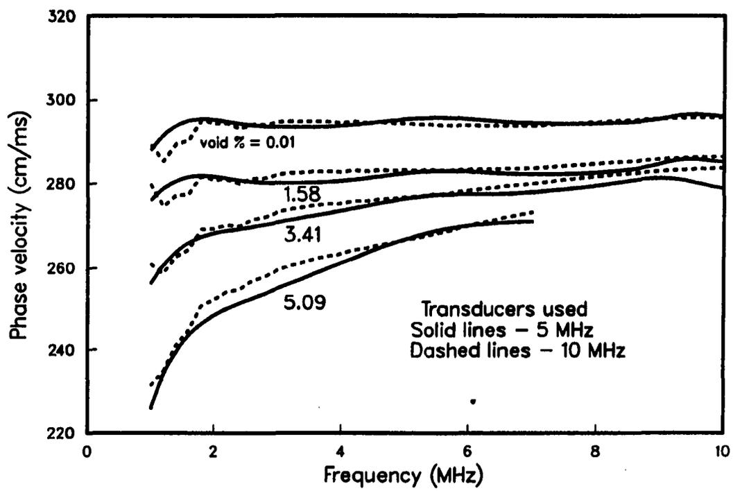
Figure 4.6: Phase velocity of longitudinal waves in woven carbon/epoxy laminates
