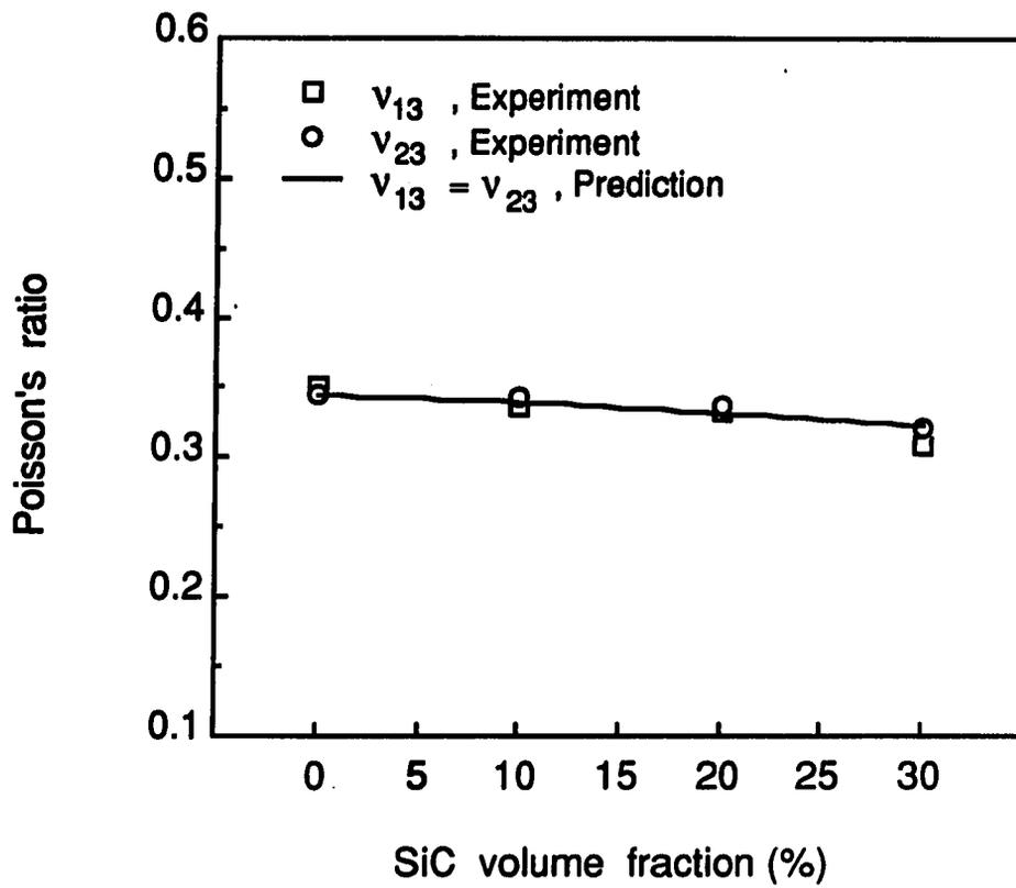
Figure 6.7: Comparison of predicted Poisson's ratios  $\nu_{13}$  and  $\nu_{23}$  with experimental results (7091 Al/SiC<sub>p</sub>)
