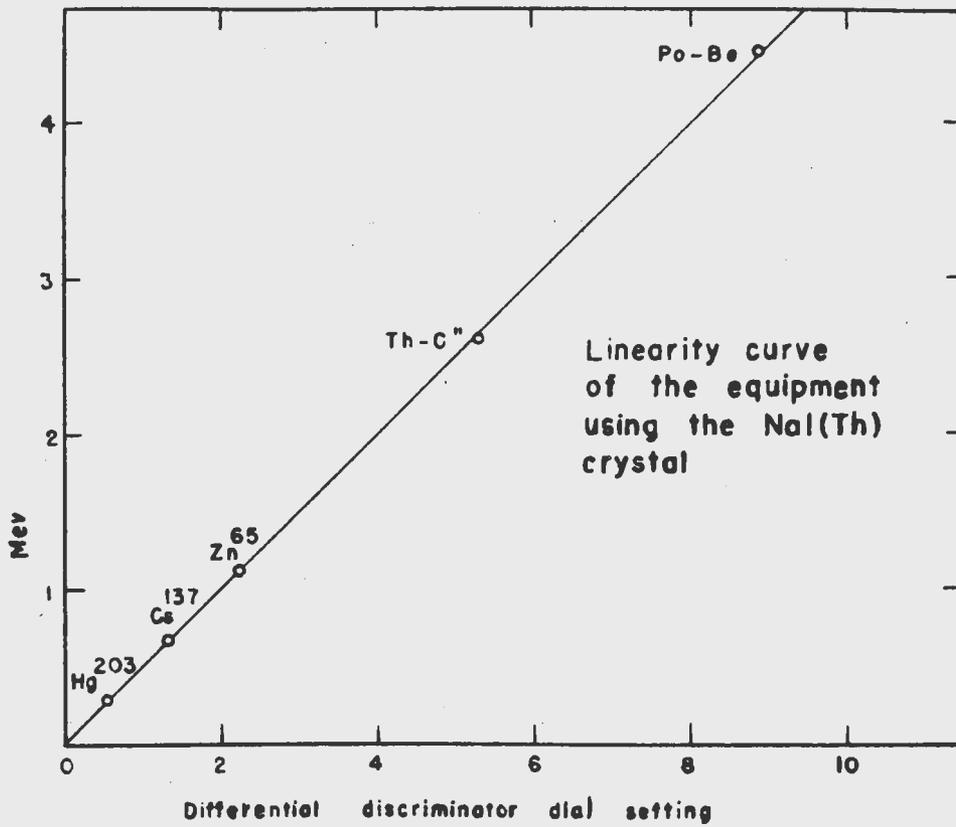
Fig. 7--Linearity test with NaI(Th) crystal.
