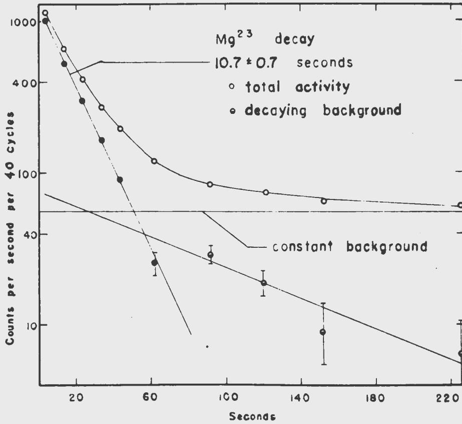
Fig. 8--Decay curve of Mg<sup>23</sup>.
