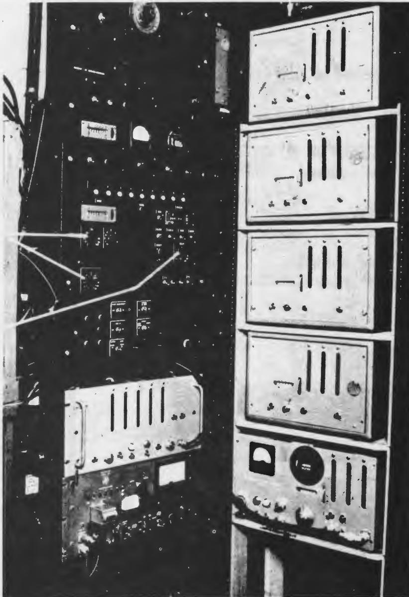
Fig. 4--Programming circuit and scaler racks.
