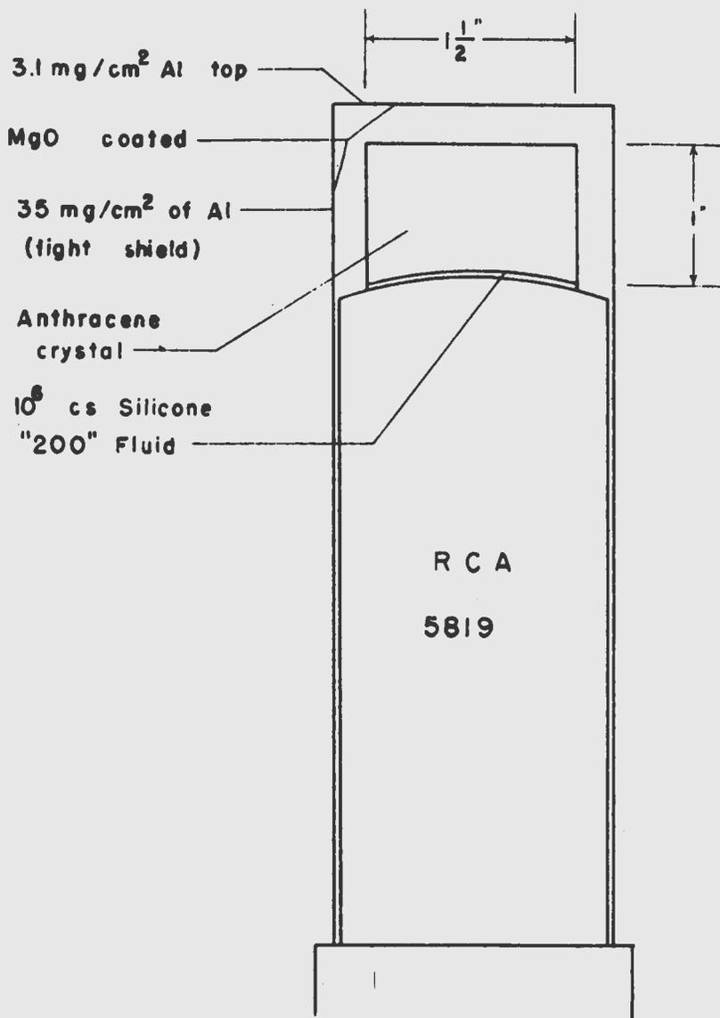
Fig. 5--Photomultiplier tube and crystal mounting.
