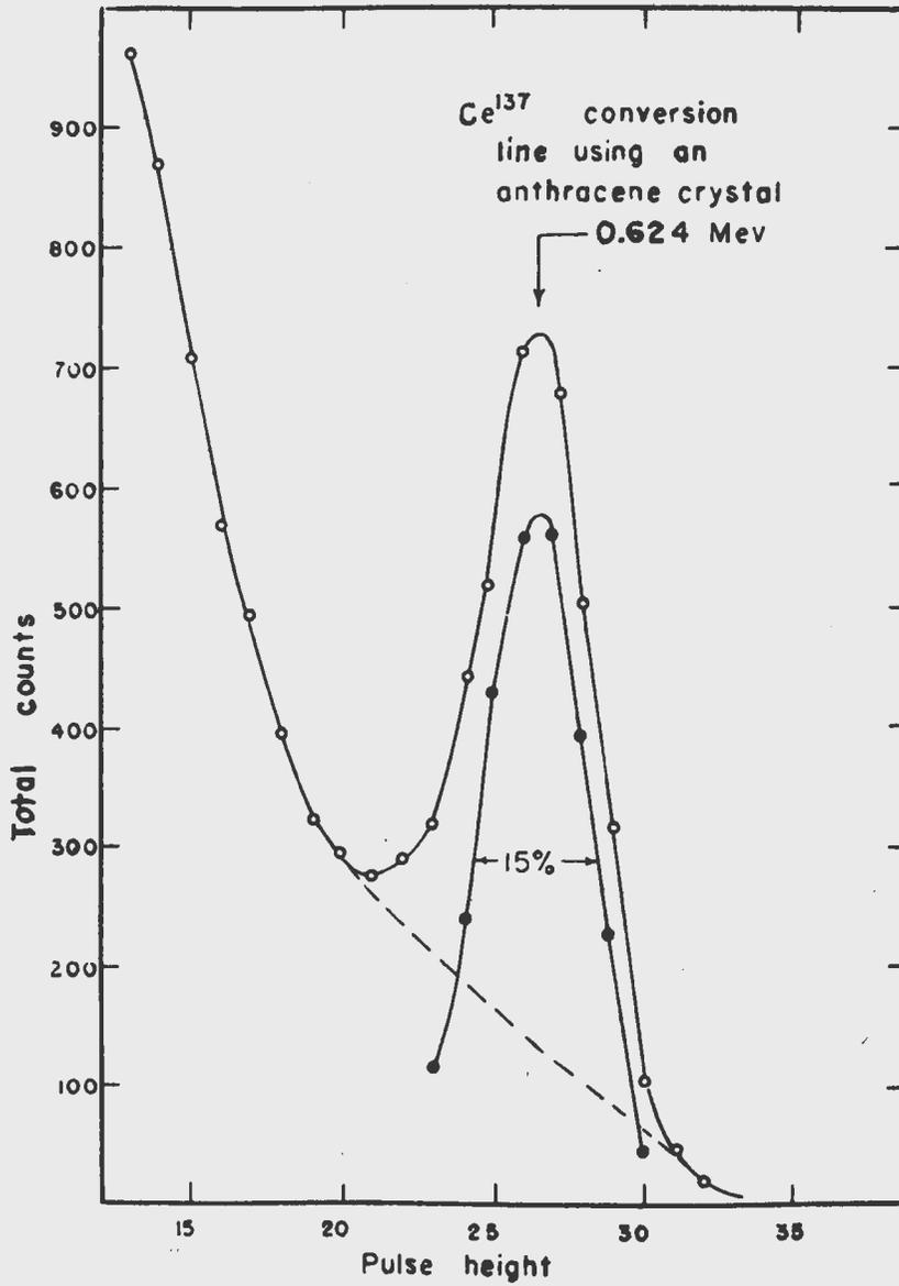
Fig. 6--Typical resolution curve for anthracene.
