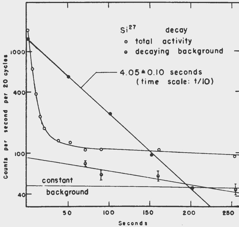
Fig. 11--Decay curve of Si<sup>27</sup>.
