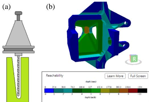
Figure 2: Reachability characteristic for machining; a) Part geometry with poor reachability, b) Color map of reachability depths
