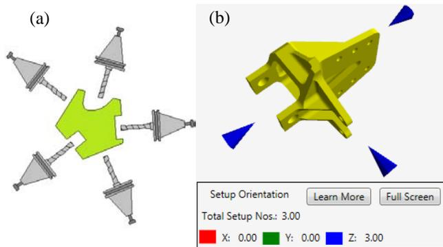
Figure 4: Setup complexity characteristic for machining; a) Geometry requiring multiple setup orientations, b) 3D representation of setup requirements
