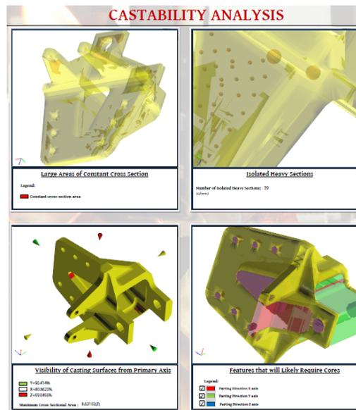
Figure 7: 3D PDF manufacturability results
