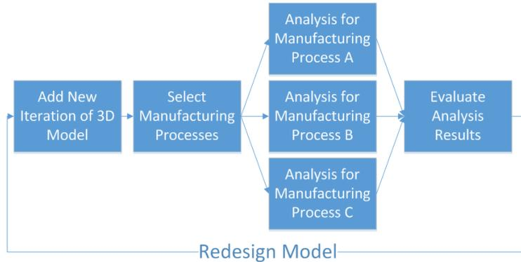
Figure 5: Information flow for automated manufacturability analysis
