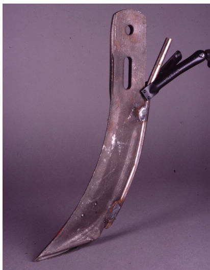
Figure 2. Knife used to inject NH 3 .
