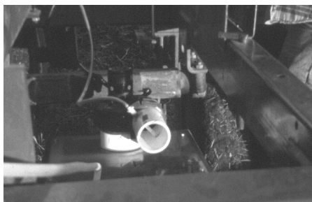
Figure 3. Top of hood over injector showing air exit from suction fan. Small tube inside air exit draws sample air used to measure NH 3 loss.
