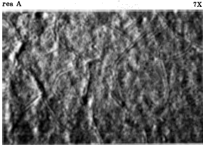
Area A Area B Fig. 6 Photomicrographs Showing Surface Condition of Two Typical Areas of As-Pressed Billet of Ceralloy 147A HPSN Where Large Numbers of Surface Wave Indications Were Detected.
