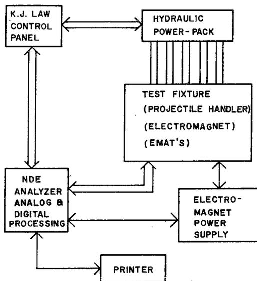
Figure 4. System block diagram.
