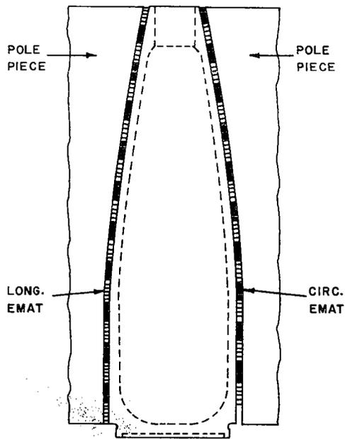
Figure 3. EMAT and pole piece configuration.
