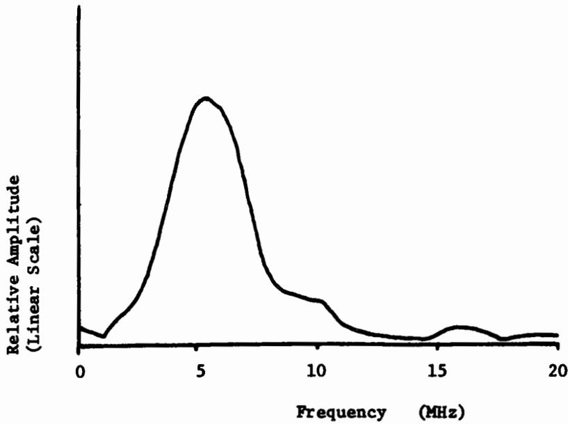
Figure 3. Fourier Transform of Input Pulse.
