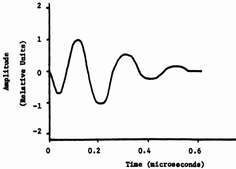
Figure 2. Ultrasonic Input Pulse.
