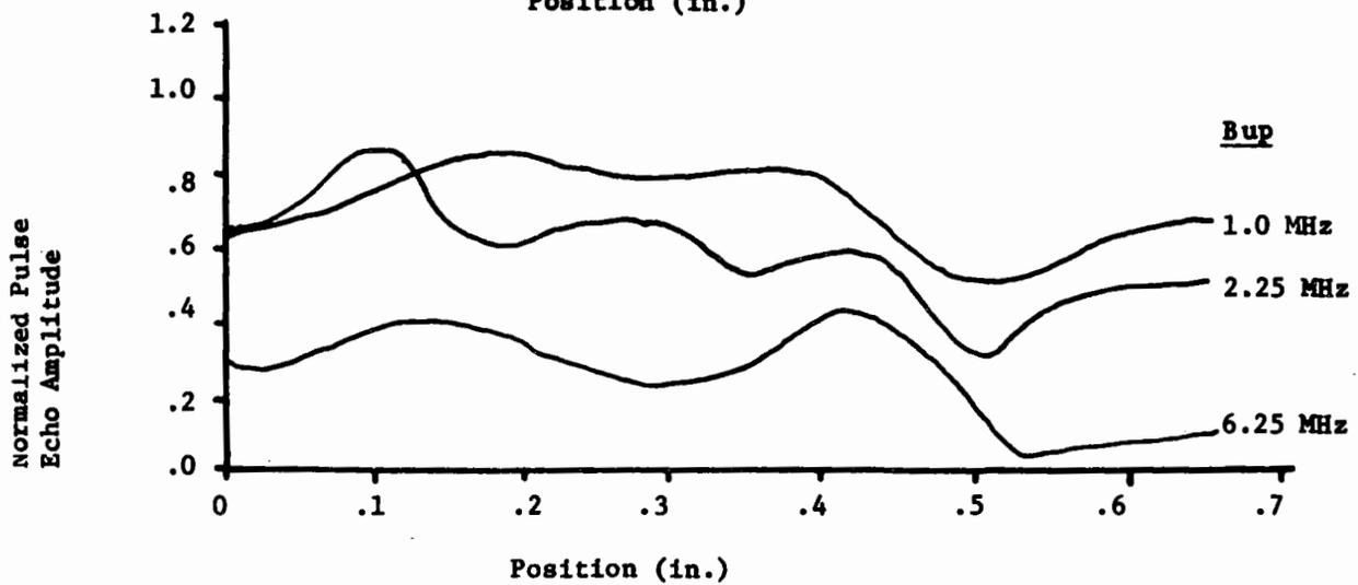
Figure 7. Reflected Ultrasonic Amplitude From Fracture Surfaces vs Position
