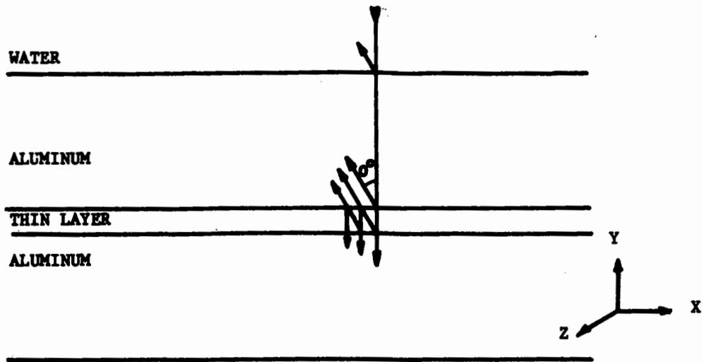
Figure 1. Schematic Illustration of Fatigue Crack Model.
