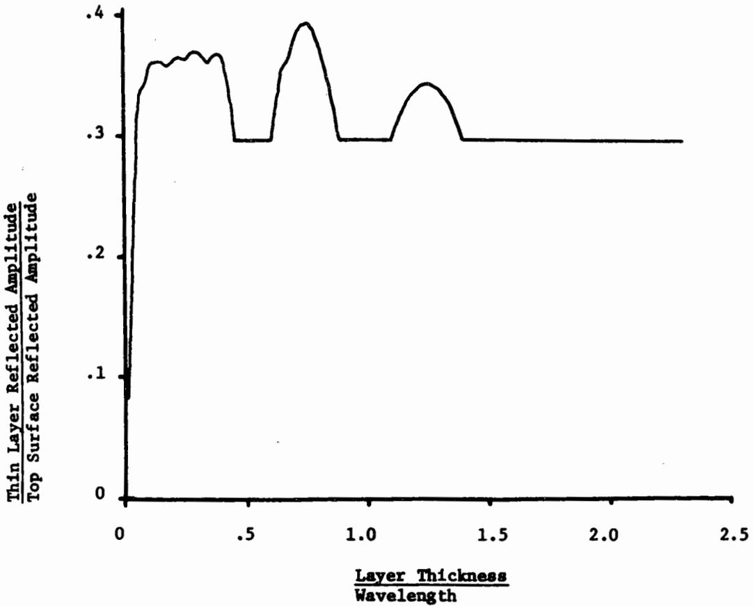
Figure 5. Peak-to-peak reflected amplitude as a function of layer thickness for a 3 cycle, 5MHz input pulse in an aluminum - water-aluminum model.
