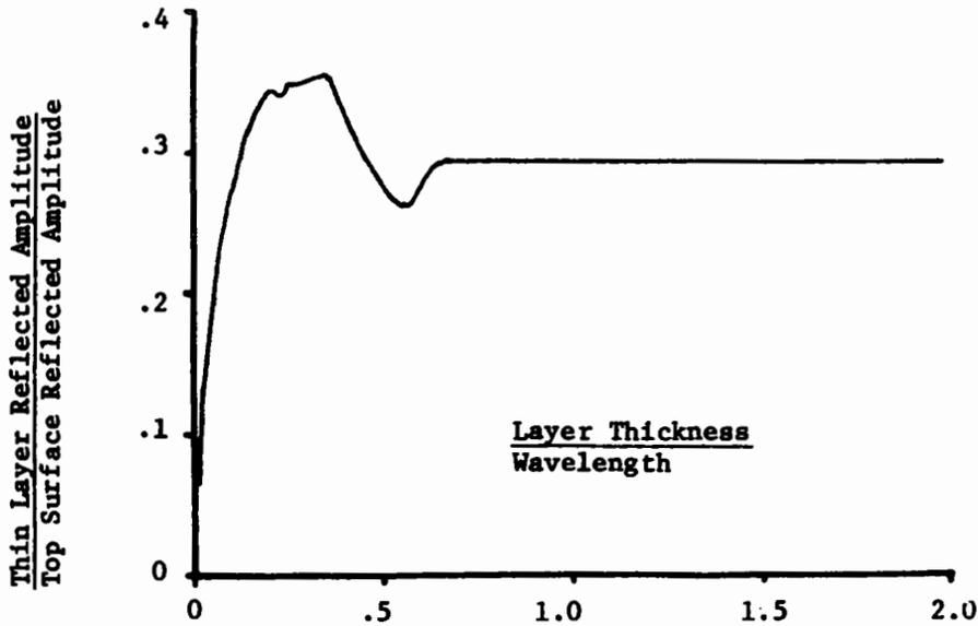
Figure 4. Peak-to-peak reflected amplitude as a function of layer thickness for input pulse in Figure 2. in an aluminum-water-aluminum model.
