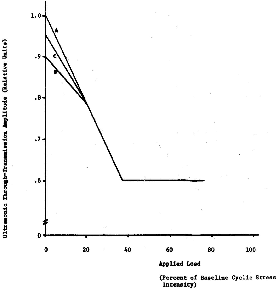
Figure 10. In Situ Through Transmission Ultrasonic Measurements in Compact Tension Specimen of 2024-T851 Aluminum Alloy.
