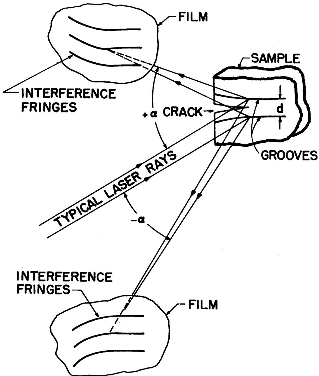
Figure 9. Schematic of the laser interferometric displacement technique.  $d$  is typically 0.51mm (0.020 in.), and  $\alpha$  is typically  $65^\circ$ .
