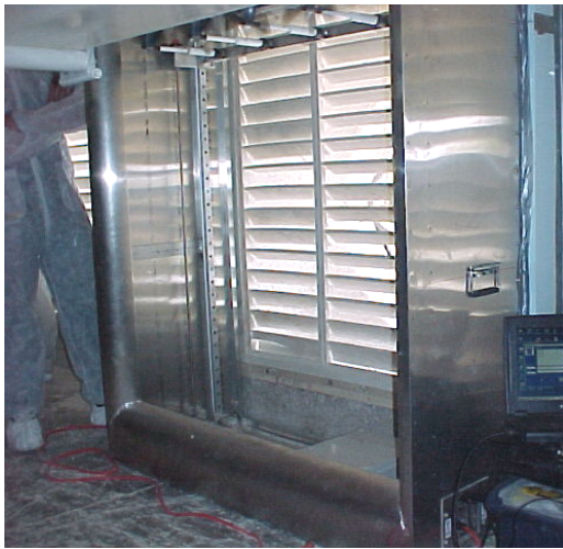
Figure 3. Snapshot of in situ calibration of airflow rate of exhaust fans in the monitored layer house using the FANS unit.
